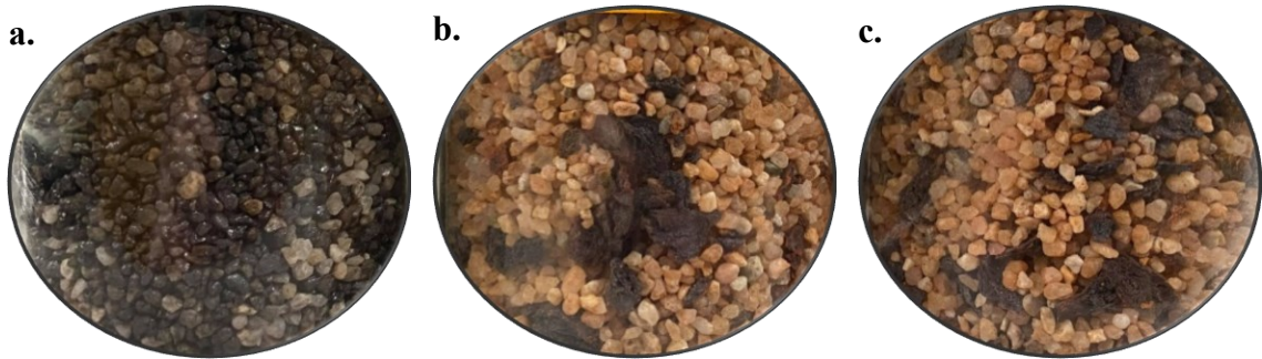
Figure D.2- 17: Experimental photos of the post-treatment ash and sand from base case I-1 from three locations within the reactor, a. the top sand cap, b. the middle of the fuel bed, and c. the bottom of the fuel bed.
