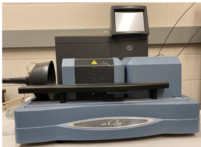
Figure 3.6 TA SDT Q600 thermogravimetric/differential scanning calorimetry analyzer.
