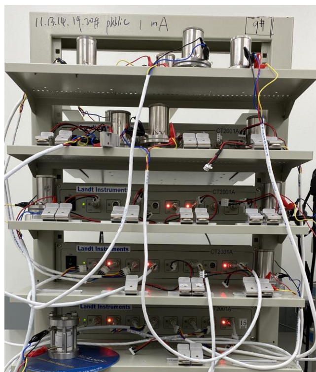
Figure 3.12 LAND CT-2001A system for SSB testing.
