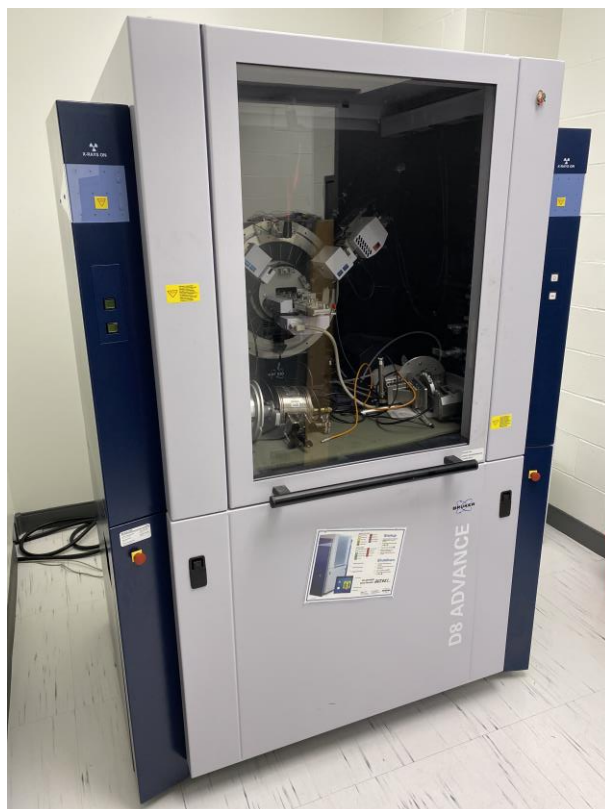
Figure 3.5 Bruker D8 Advance Diffractometer XRD system.
