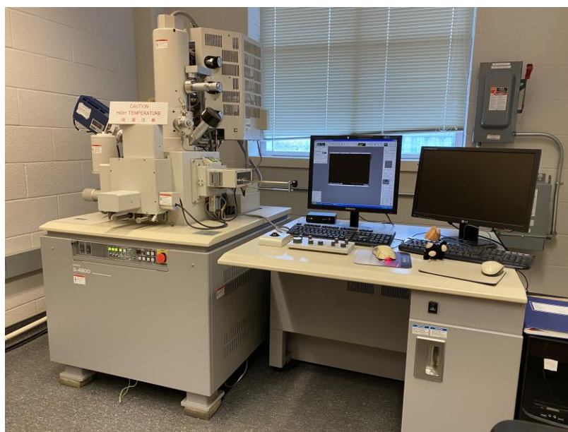
Figure 3.3 Hitachi S4800 scanning electron microscopy.
