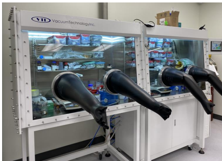
Figure 3.10 Photo of glove box for battery assembling.
