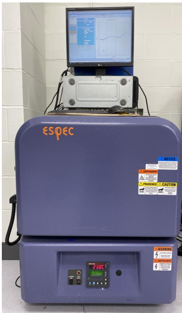
Figure 3.13 Multichannel potentiostat 3/Z (VMP3) system and the oven for temperature testing.
