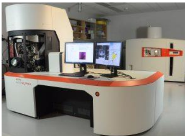
Figure 3.8 Kratos AXIS Nova (rear) X-ray photoelectron spectrometers at Surface Science Western.
