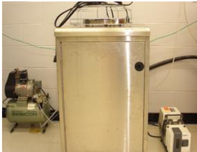
Figure 3.1 Savannah 100 ALD system (Ultratech/Cambridge Nanotech., USA)
