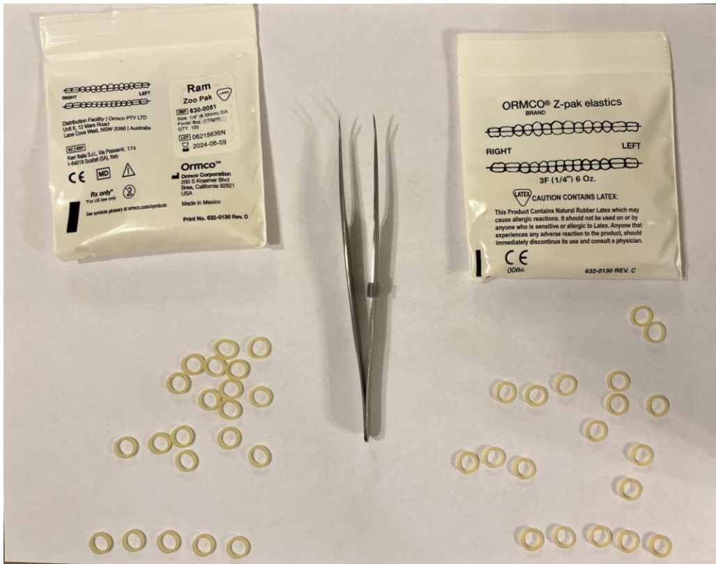
Figure 5: Ten elastics total (five elastics from each of the manufacturer’s two separate lots) were selected for testing after being visually inspected.
