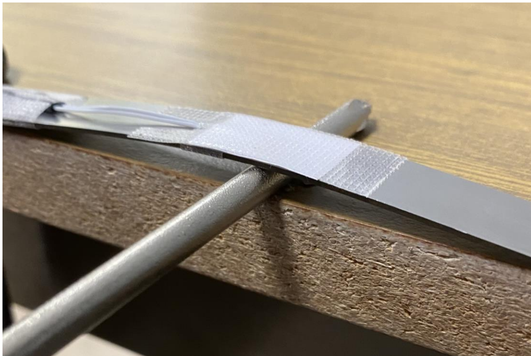
Figure B.3: Beam deflection using a 0.7 mm diameter rod for strain measurement
