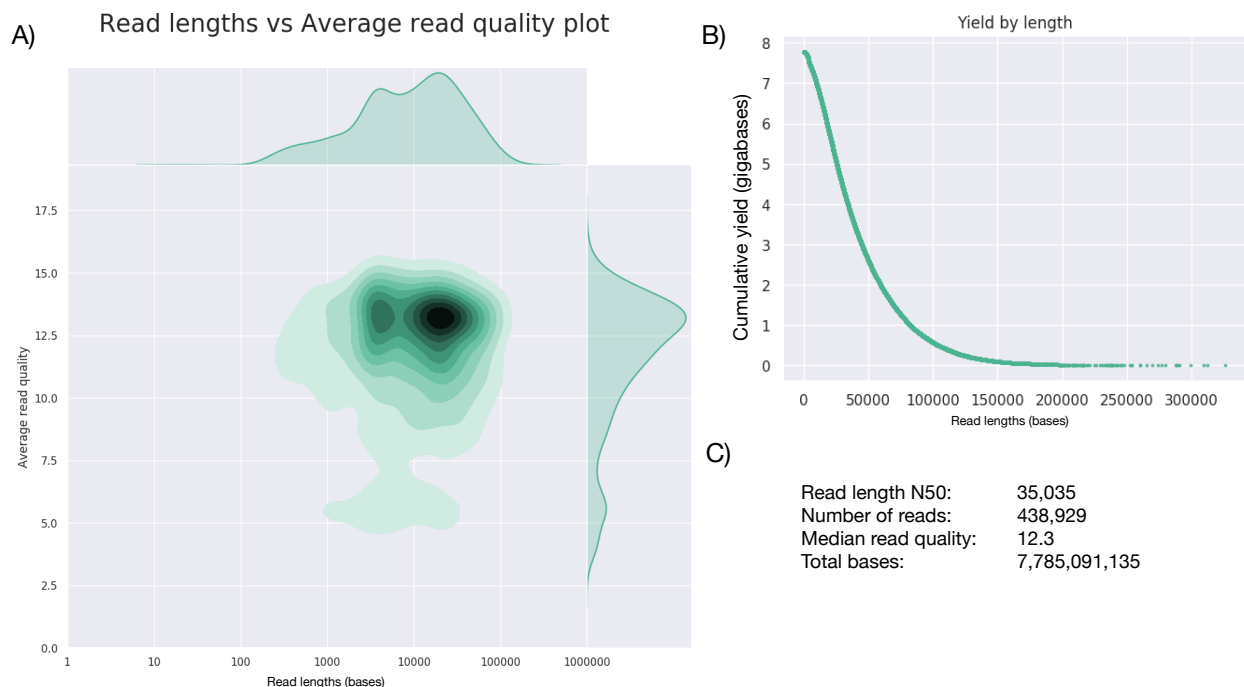
Figure 3.1: Quality characteristics of ultra-long sequencing run generated by NanoPlot (11). A) Density plot of read length vs average Q score per read. B) Yield by read length. The cumulative yield refers to the total number of bases on a sequencing read larger than the denoted number on the x-axis. C) Various quality statistics.
