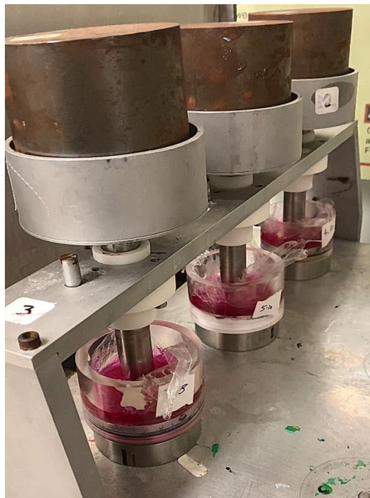
Figure 2-4: Wear testing set up.
