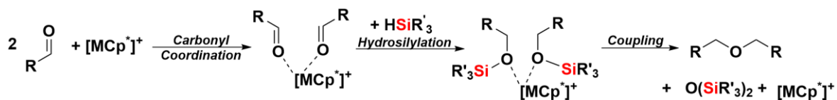
Scheme 5.3 Proposed pathway for the formation of symmetric ethers from aldehydes and silanes catalyzed by [\text{MCp}^*][\text{B}(\text{C}_6\text{F}_5)_4] . 5
