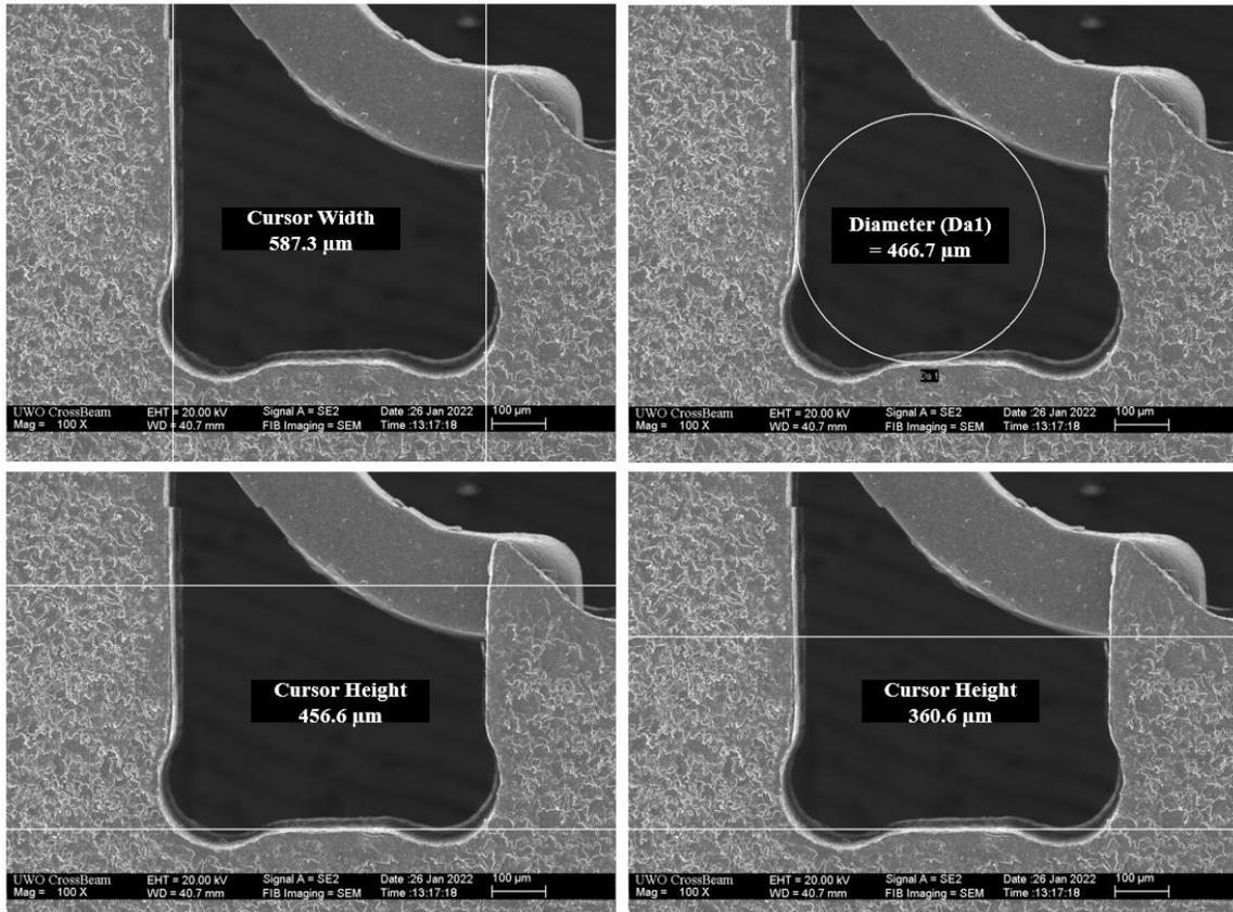
**Appendix D: Scanning electron microscopy images of A-Vic brackets with various measurements and included reference points from which measurements were made. Magnification and image scale is included in each individual image. Measures are reported in  $\mu\text{m}$ , where  $1\mu\text{m} = 0.0397\text{mils}$**
