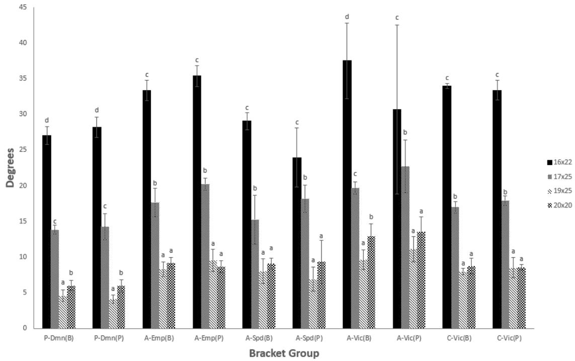
**Figure 36: Mean engagement angles in degrees ( $\pm$ SD) with different wire sizes (mil) versus bracket system. Error bars represent 1 SD, and letters shared within each bracket group cluster represent non-significant differences between wire sizes at  $P > 0.05$**
