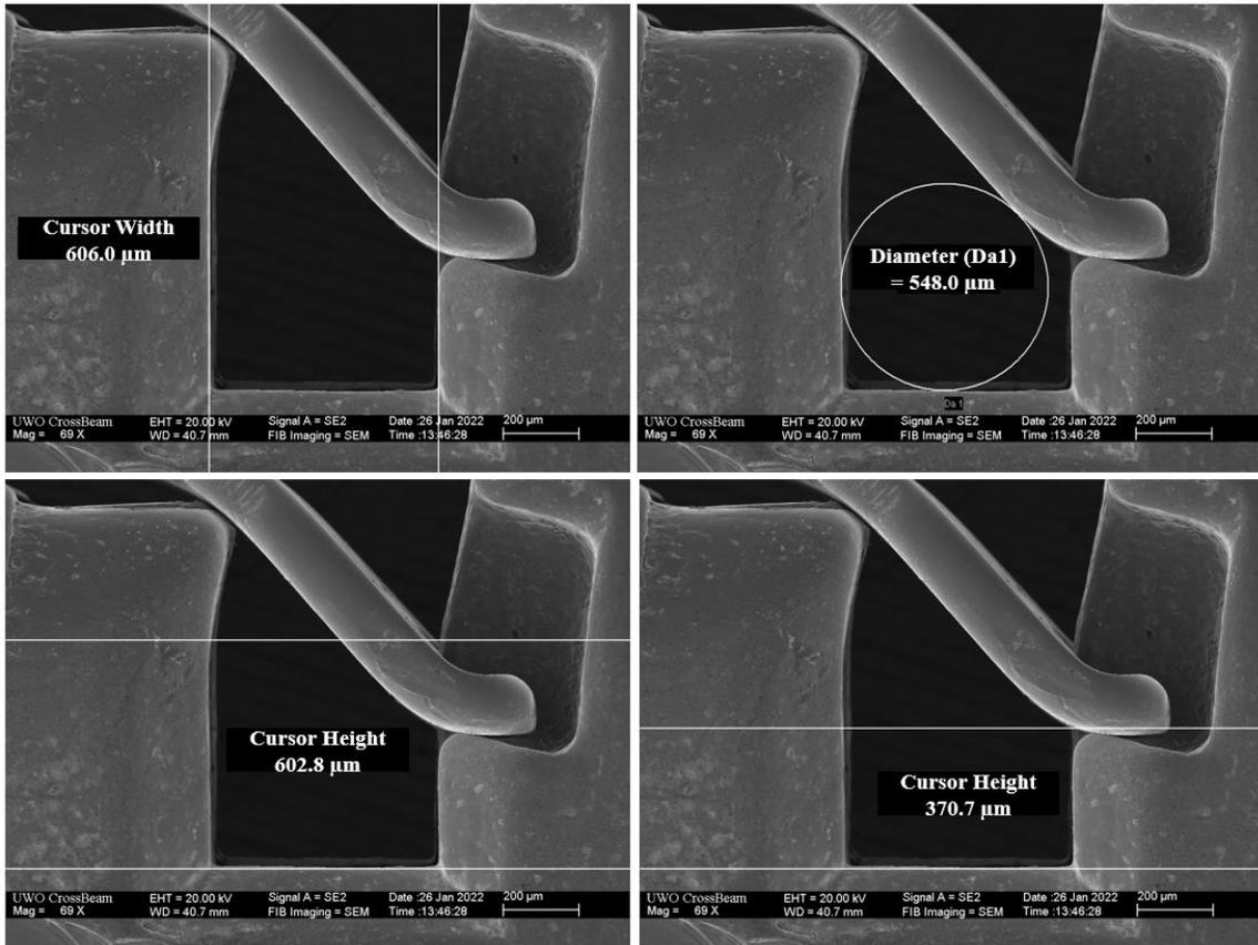
**Appendix C: Scanning electron microscopy images of A-Spd brackets with various measurements and included reference points from which measurements were made. Magnification and image scale is included in each individual image. Measures are reported in  $\mu\text{m}$ , where  $1\mu\text{m} = 0.0397\text{mils}$**
