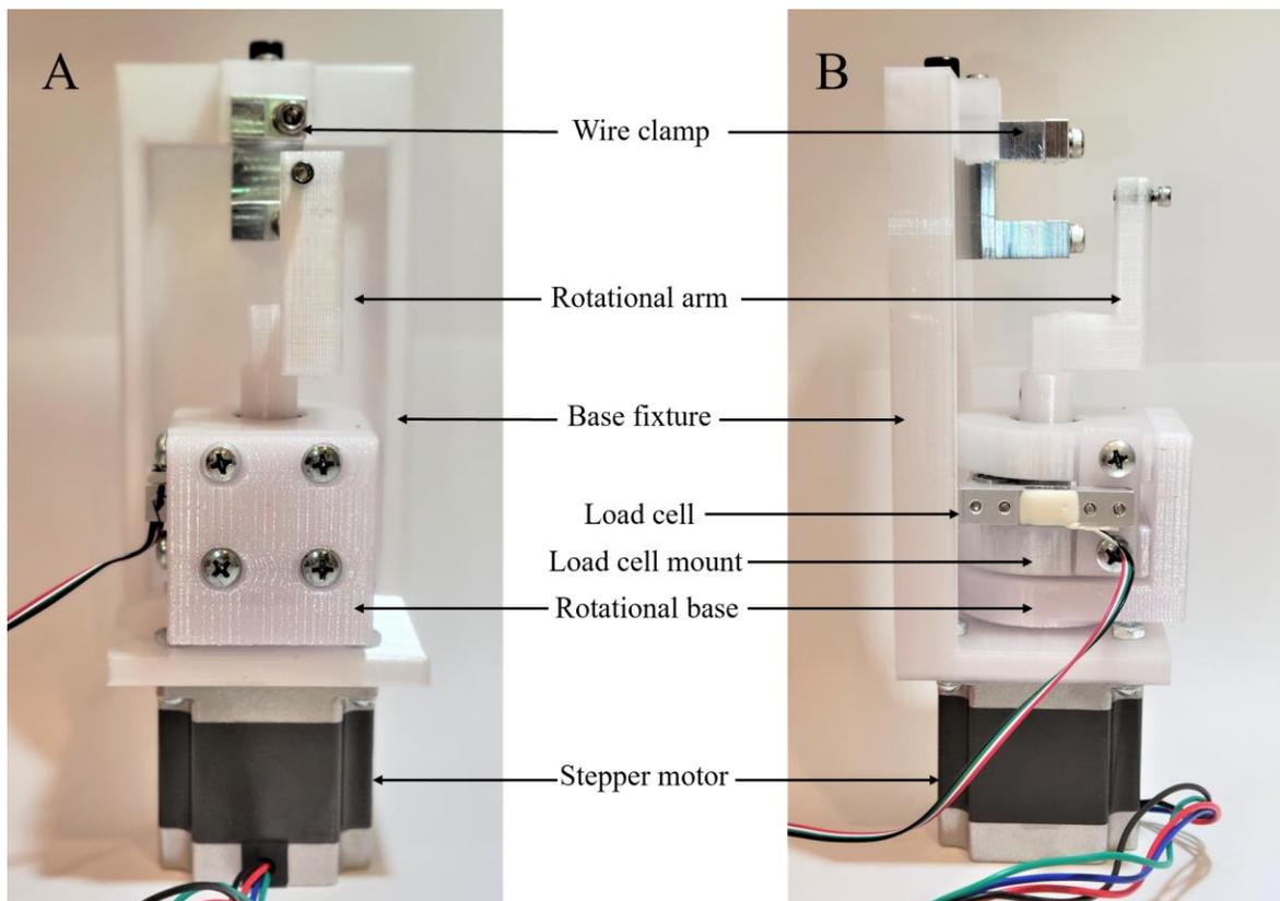
**Figure 16: Custom torque assembly as viewed from the front (A) and side (B) perspectives. Labels highlight the main components of the assembly: the stepper motor, torque-measuring fixture (load cell and load cell mount mounted on a rotational base), rotational arm, and base fixture with wire clamps**
