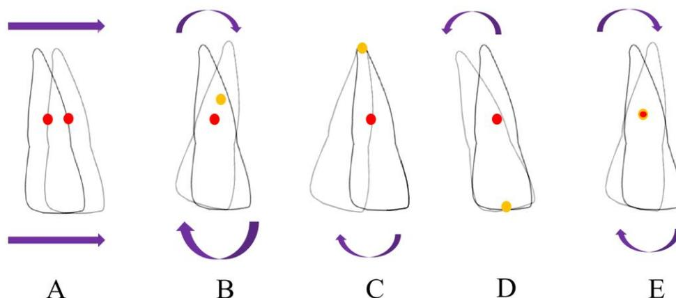
**Figure 5: Categories of orthodontic tooth movement, including translation (A), uncontrolled tipping (B), controlled tipping (C), root movement (D), and pure rotation (E). Red dots represent the center of resistance while orange dots represent the center of rotation**
