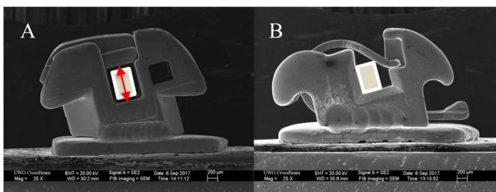
**Figure 12: Scanning electron microscopy images of a passive (A) and active (B) SL bracket. The former highlights the door-type mechanism providing freedom to the wire within the slot, while the latter demonstrates the active clip mechanism seating the wire within the bracket slot. Image used with permission from a previous thesis completed by Greene et al<sup>75</sup>©**
