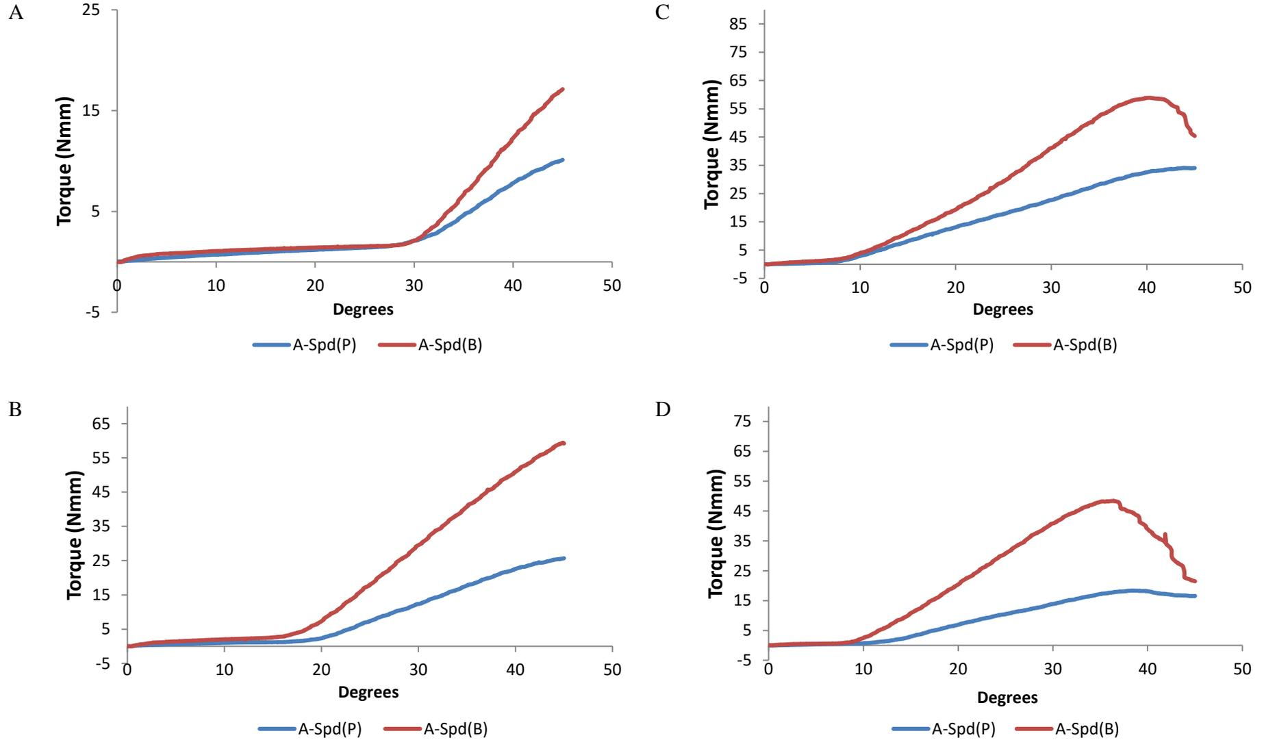
**Figure 32: Mean torquing moments measured for A-Spd brackets in both buccal (A-Spd(B)) and palatal (A-Spd(P)) root torque simulation directions with 16 x 22 mil SS wire (A), 17 x 25 mil SS wire (B), 19 x 25 mil SS wire (C), and 20 x 20 mil SS wire (D)**
