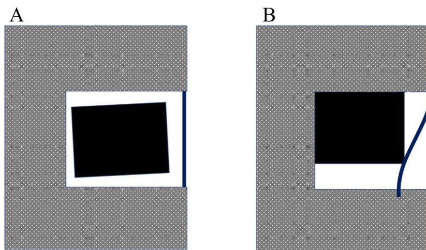
**Figure 39: PSL and ASL start position diagrams. (A) demonstrates that a PSL system can have some degree of wire twist while appearing in a zero initial position, while (B) demonstrates ASL systems have a more repeatable initial starting zero position. The grey patterned area represents the bracket, black represents a wire engaged in the slot, as viewed in cross-section**
