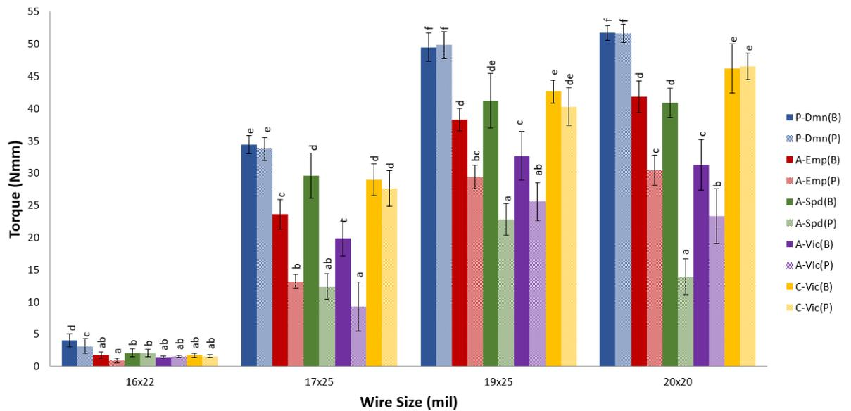
**Figure 25: Mean torquing moments in Nmm ( $\pm$ SD) measured at 30 degrees with different bracket systems versus wire size. Error bars represent 1 SD, and letters shared within each wire size cluster represent non-significant differences between bracket systems at  $P > 0.05$**
