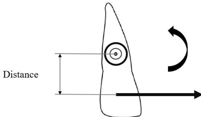
**Figure 3: A force applied a distance from the Center of Resistance will tend to produce rotation. The tendency to produce rotation is known as Moment of the Force, which is equal to the magnitude of the force multiplied by the distance between the Line of Action of the force and the Center of Resistance of the object**
