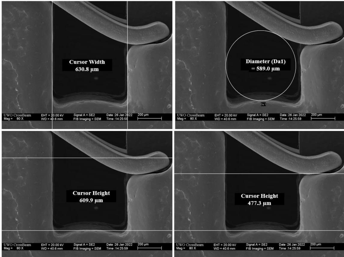
**Appendix E: Scanning electron microscopy images of C-Vic brackets with various measurements and included reference points from which measurements were made. Magnification and image scale is included in each individual image. Measures are reported in  $\mu\text{m}$ , where  $1\mu\text{m} = 0.0397\text{mils}$**
