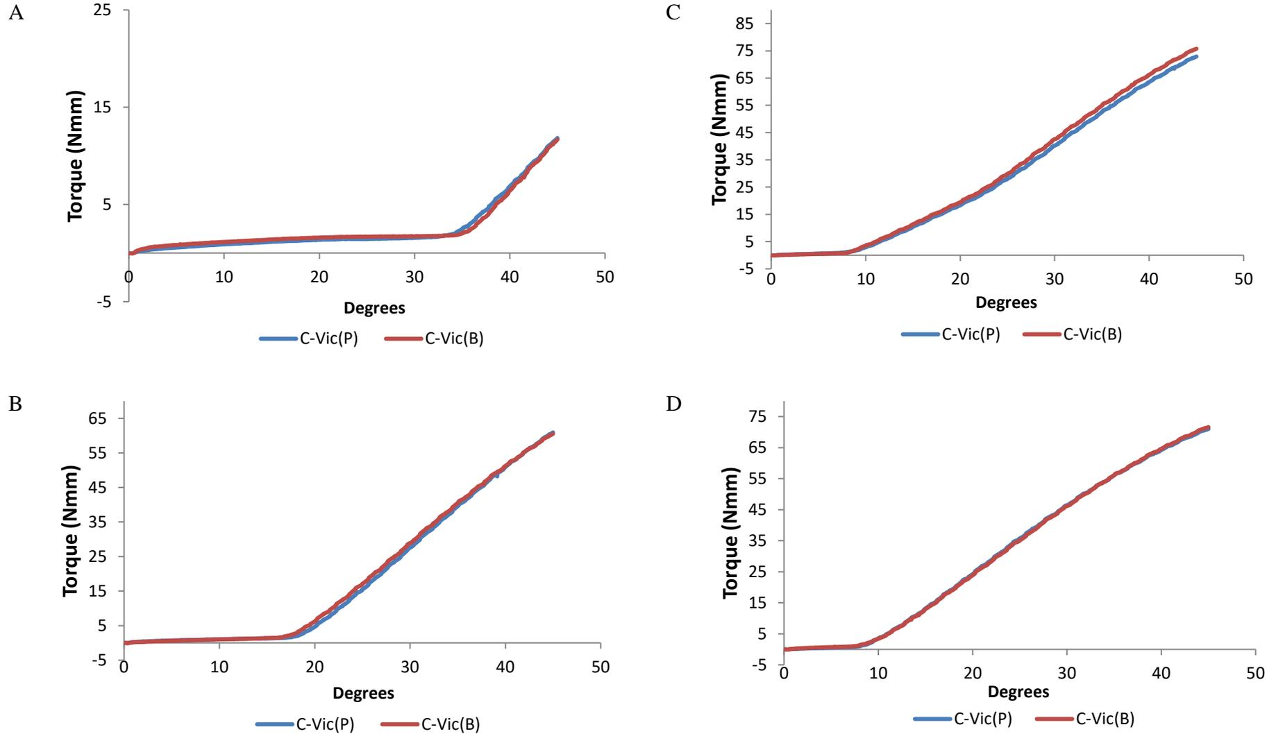
**Figure 34: Mean torquing moments measured for C-Vic brackets in both buccal (C-Vic(B)) and palatal (C-Vic(P)) root torque simulation directions with 16 x 22 mil SS wire (A), 17 x 25 mil SS wire (B), 19 x 25 mil SS wire (C), and 20 x 20 mil SS wire (D)**
