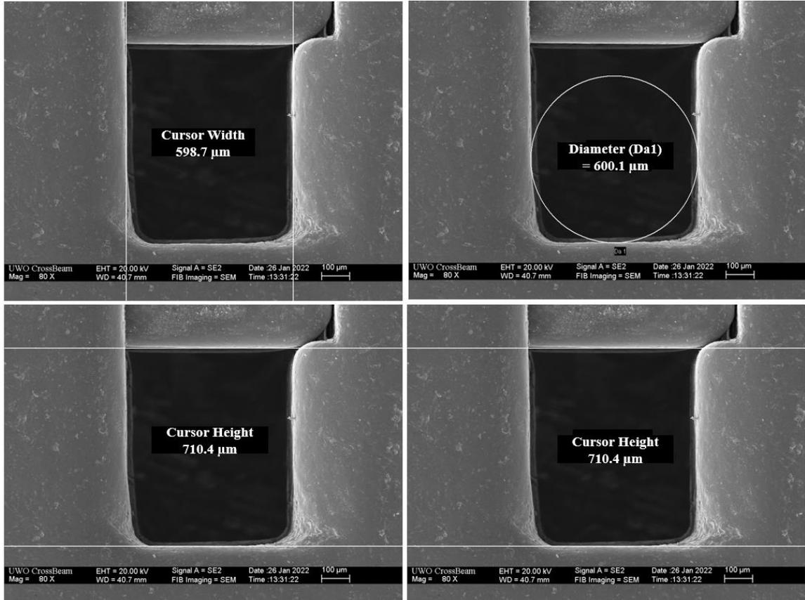
**Appendix B: Scanning electron microscopy images of A-Emp brackets with various measurements and included reference points from which measurements were made. Magnification and image scale is included in each individual image. Measures are reported in  $\mu\text{m}$ , where  $1\mu\text{m} = 0.0397\text{mils}$**
