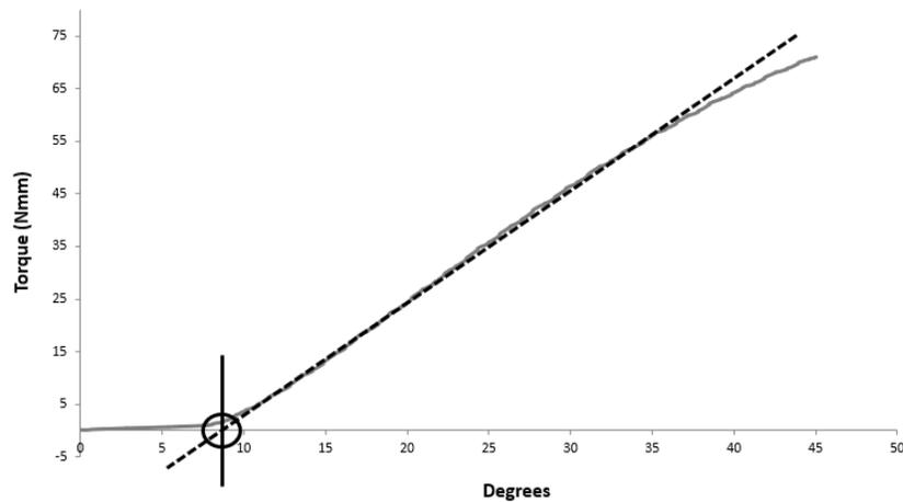
**Figure 19: To determine engagement angle, a line was fit to the linear portion of the mean torque-rotation curve by computer code and the angle at which this line passed through zero was assigned as the engagement angle**
