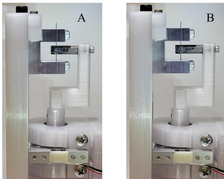
**Figure 18: Brackets mounted in the custom torque assembly with the gingival oriented downward relative to the mounting jig to simulate buccal root torque (A), and the gingival oriented upward relative to the mounting jig to simulate palatal root torque (B)**
