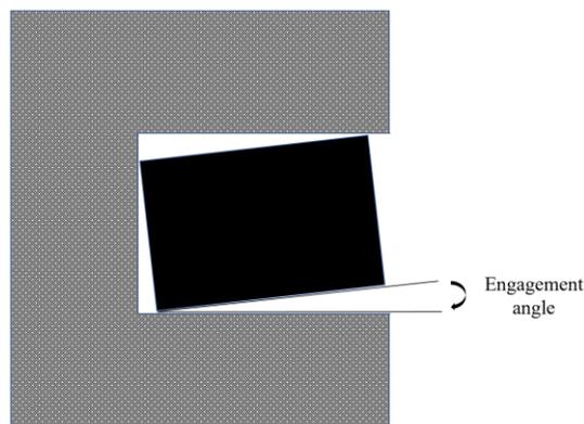
**Figure 9: Pictorial representation of a cross-section of wire twisting within a bracket slot, as viewed from a mesial or distal view of the bracket. The grey patterned area represents the bracket, black represents a wire engaged in the slot. Engagement angle is outlined within the image**
