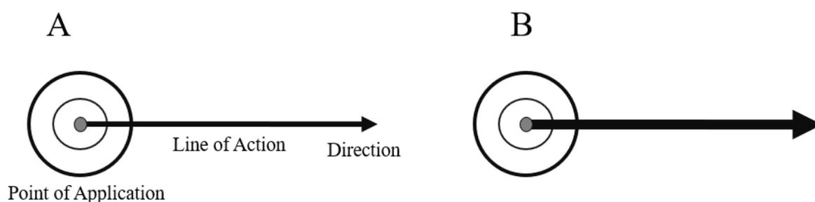
**Figure 1: Forces are vectors characterized by a point of application, line of action, and direction. Magnitude may be indicated by thickness of the force vector, with (A) demonstrating a smaller force and (B) a larger force**
