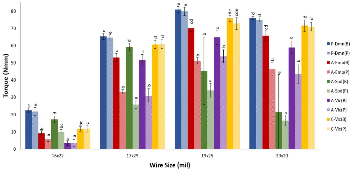
**Figure 26: Mean torquing moments in Nmm ( $\pm$ SD) measured at 45 degrees with different bracket systems versus wire size. Error bars represent 1 SD, and letters shared within each wire size cluster represent non-significant differences between bracket systems at  $P > 0.05$**
