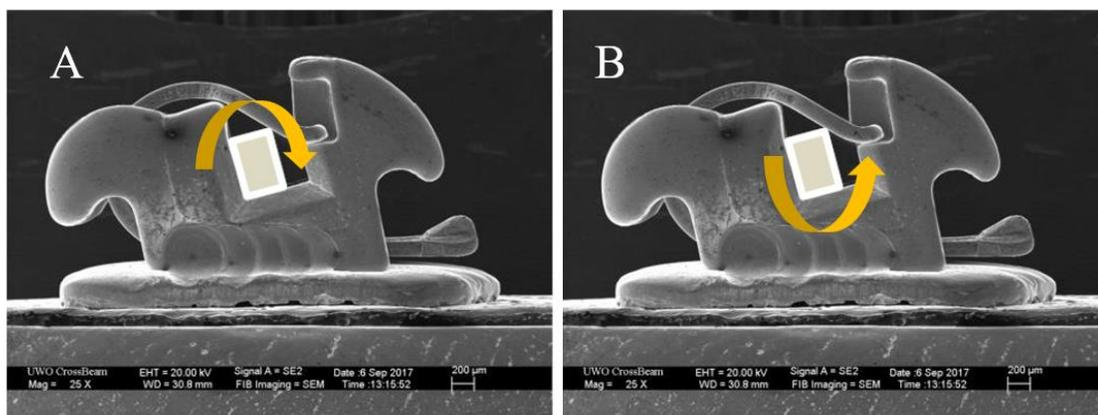
**Figure 38: Scanning electron microscopy view of a self-ligating bracket, demonstrating the discrepancy in slot depth between incisal and gingival aspects to allow for seating of the active clip. (A) demonstrates the wire twist required to generate palatal root torque, (B) demonstrates the wire twist required to generate buccal root torque. Image used with permission from previous thesis completed by Greene et al<sup>75</sup>©**
