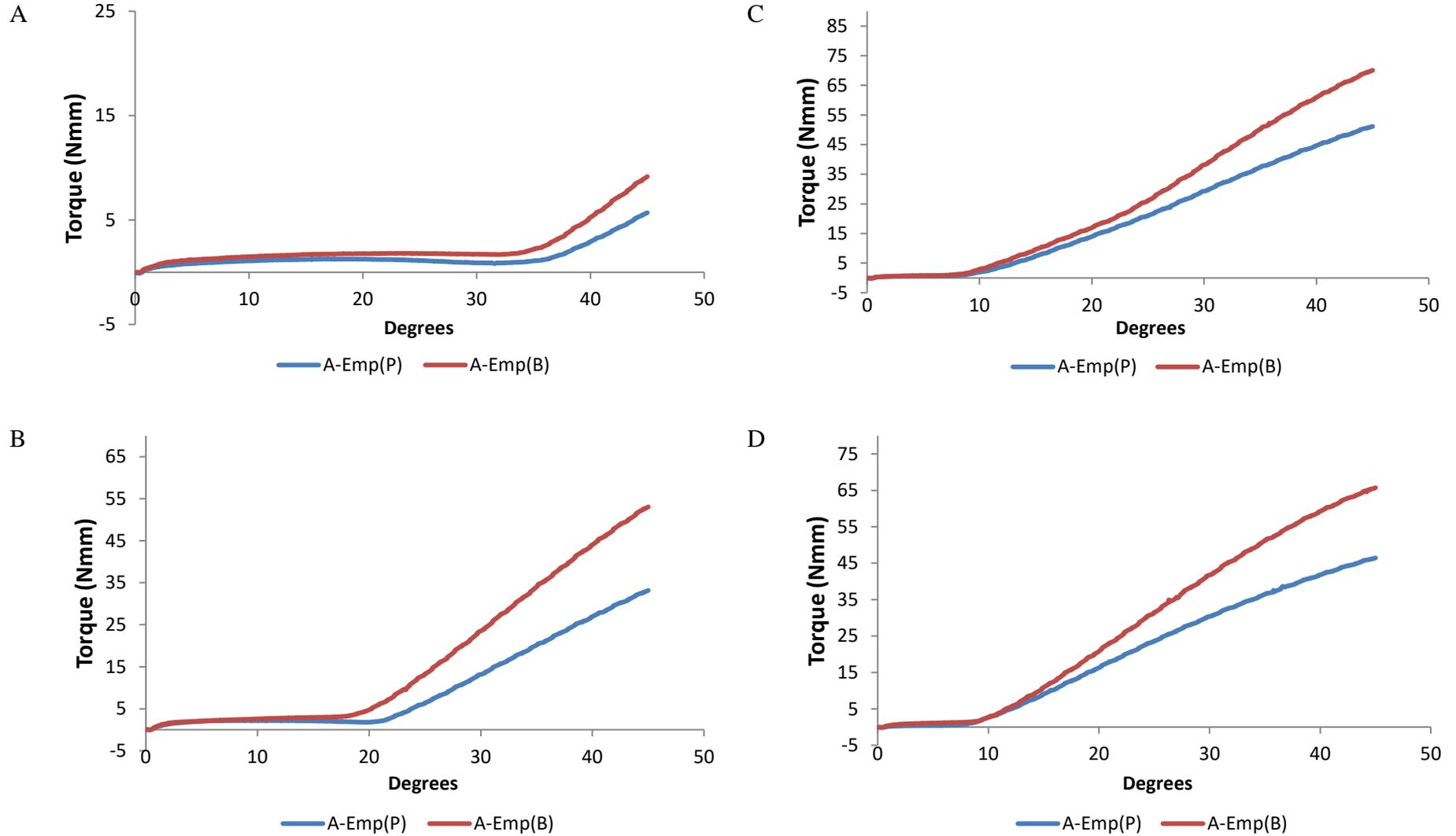
**Figure 31: Mean torquing moments measured for A-Emp brackets in both buccal (A-Emp(B)) and palatal (A-Emp(P)) root torque simulation directions with 16 x 22 mil SS wire (A), 17 x 25 mil SS wire (B), 19 x 25 mil SS wire (C), and 20 x 20 mil SS wire (D)**
