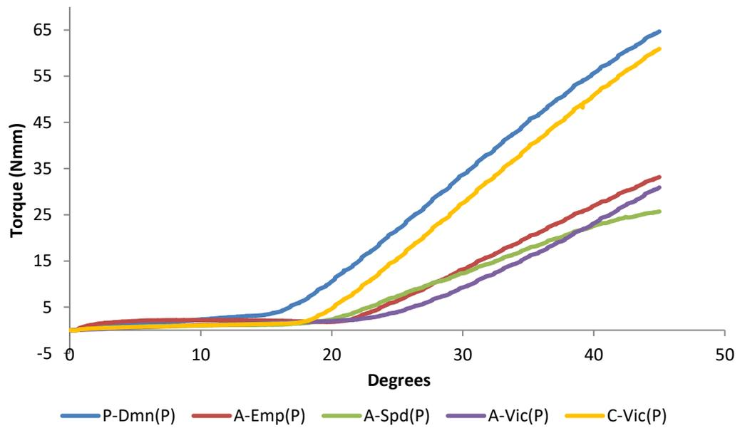
**Figure 21: Mean torquing moments measured for each bracket system and 17 x 25 mil SS wires, simulating both buccal (A) and palatal root torque (B)**
