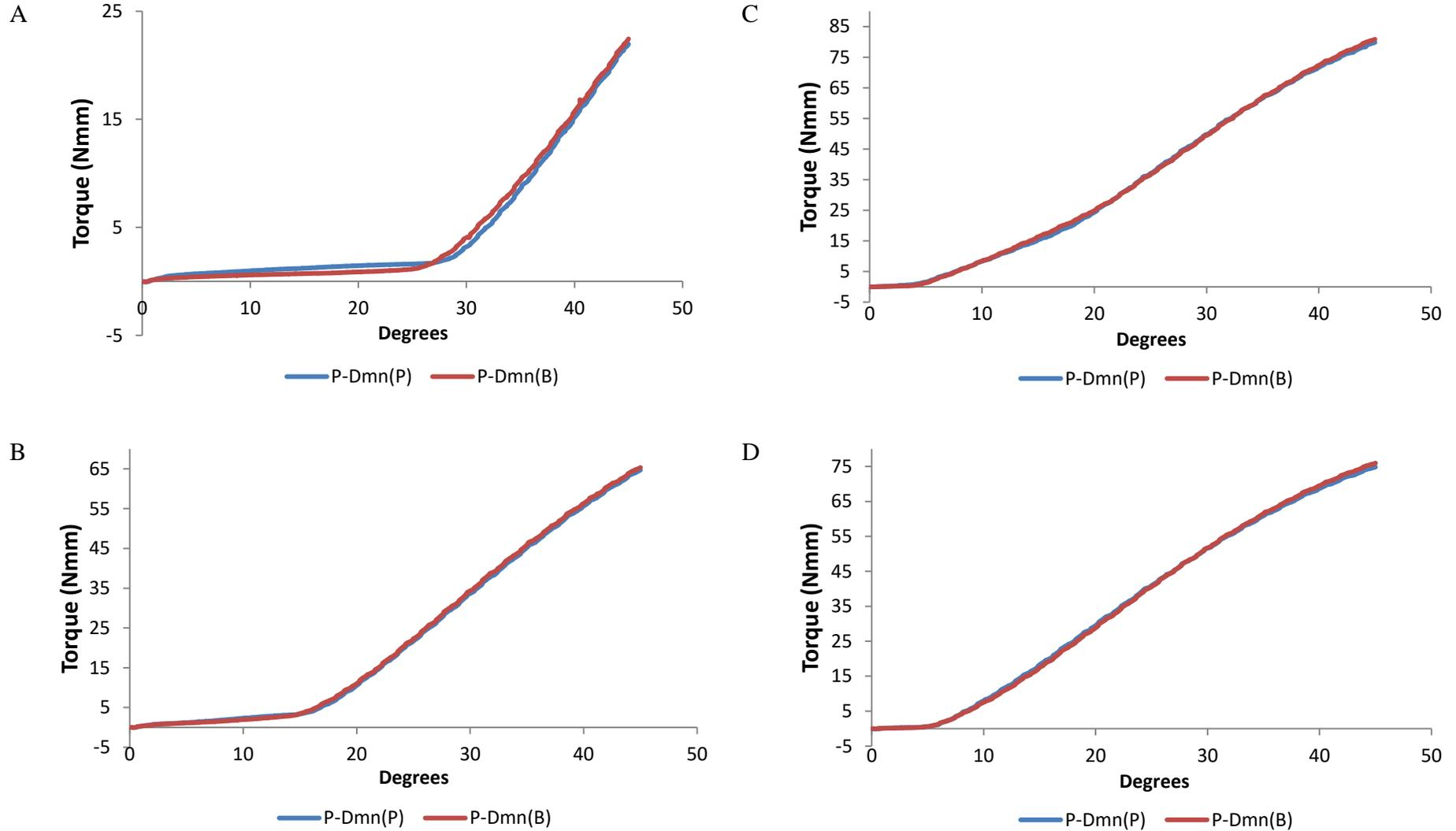
**Figure 30: Mean torquing moments measured for P-Dmn brackets in both buccal (P-Dmn(B)) and palatal (P-Dmn(P)) root torque simulation directions with 16 x 22 mil SS wire (A), 17 x 25 mil SS wire (B), 19 x 25 mil SS wire (C), and 20 x 20 mil SS wire (D)**
