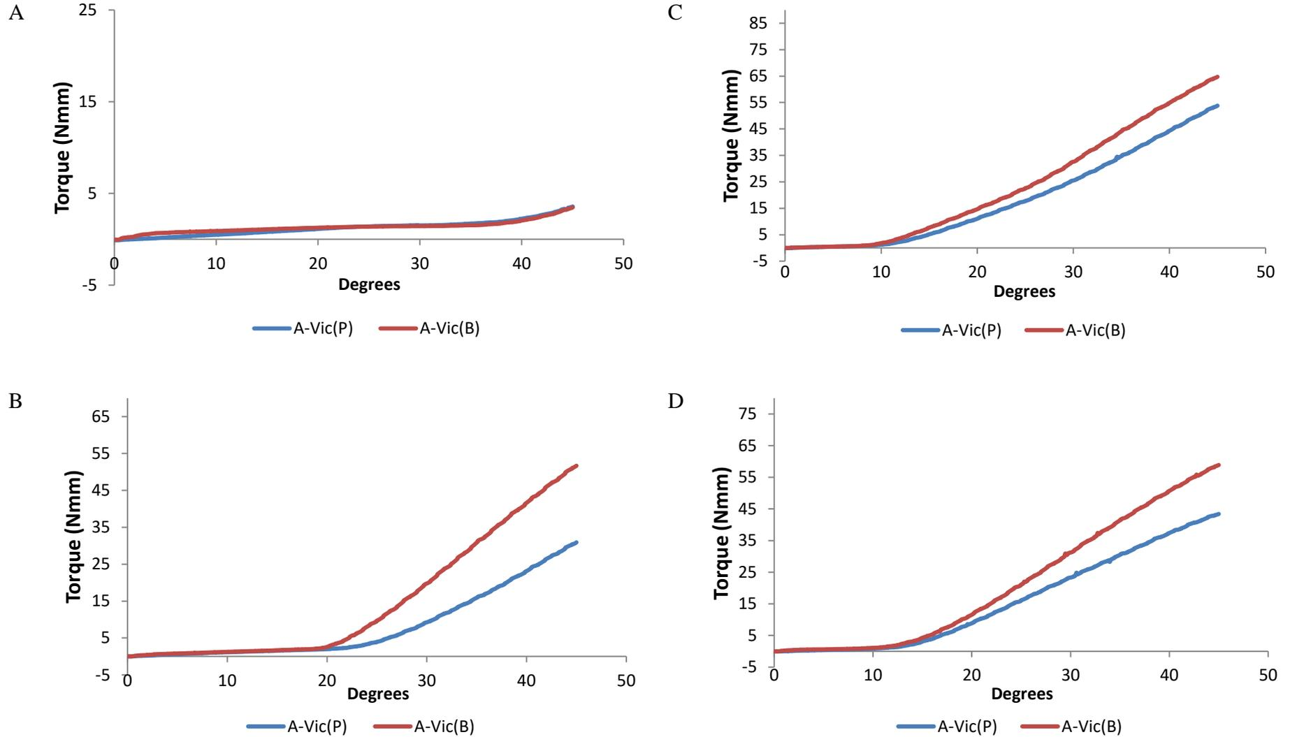
**Figure 33: Mean torquing moments measured for A-Vic brackets in both buccal (A-Vic(B)) and palatal (A-Vic(P)) root torque simulation directions with 16 x 22 mil SS wire (A), 17 x 25 mil SS wire (B), 19 x 25 mil SS wire (C), and 20 x 20 mil SS wire (D)**
