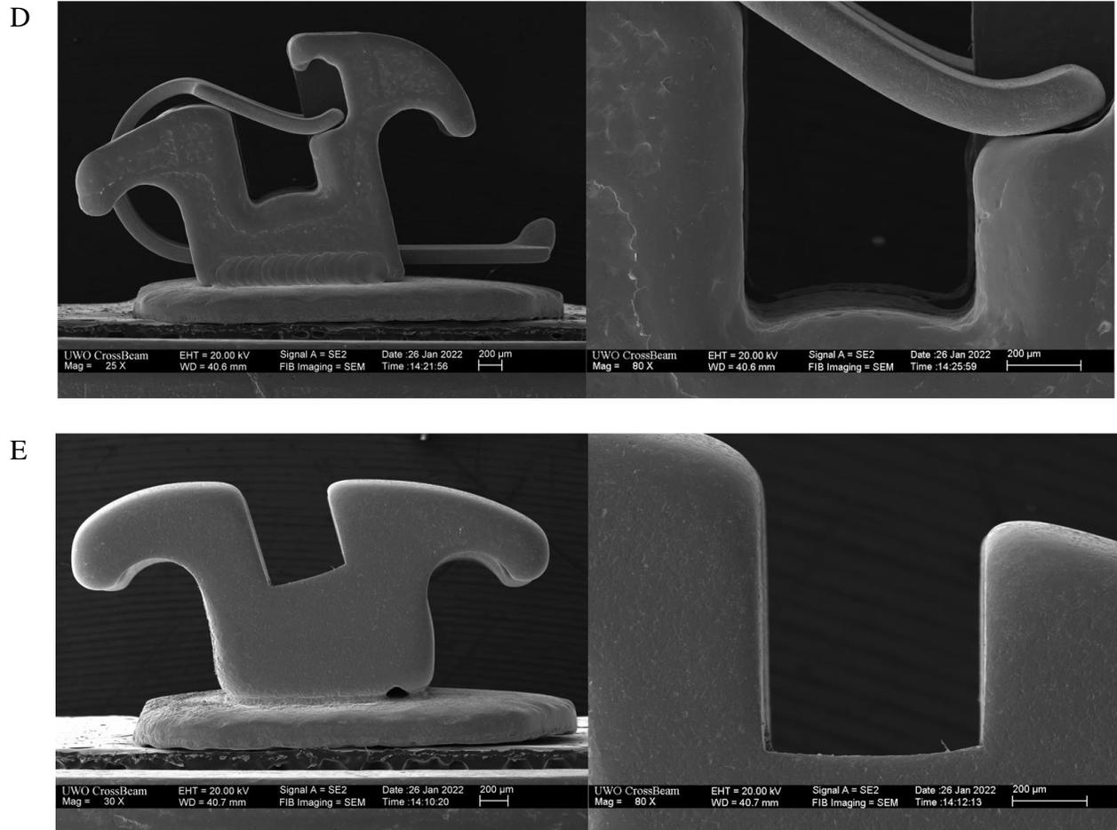
**Figure 13: Scanning electron microscopy images of each bracket system of interest, with (A) showing P-Dmn, (B) A-Emp, (C) A-Spd, (D) A-Vic, (E) C-Vic. Leftward images represent the entire bracket with the gingival aspect oriented rightward, rightward images represent a magnified image of the bracket slot itself. Magnification and references scales are shown on each individual image. Various measurements obtained within the bracket slot are found in Appendices A-E**
