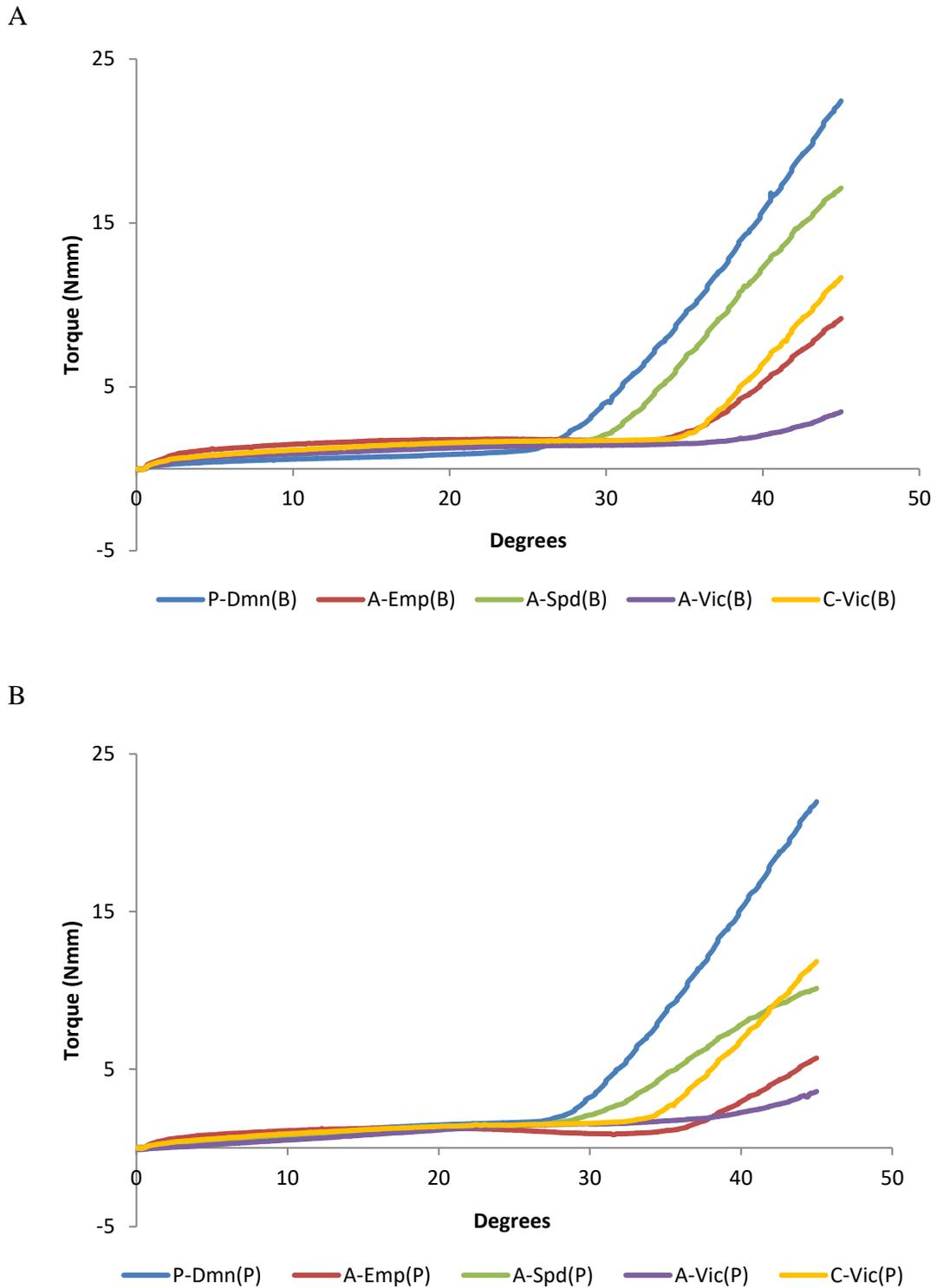
**Figure 20: Mean torquing moments measured for each bracket system and 16 x 22 mil SS wires, simulating both buccal (A) and palatal root torque (B)**
