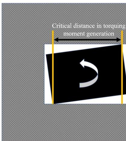
**Figure 37: Critical distance in torquing moment generation, as per the formula  $\text{Moment of a couple} = \text{Force} \times \text{Distance}$ . The grey patterned area represents the bracket as viewed in cross section, black represents a wire engaged in the slot, as viewed in cross-section**
