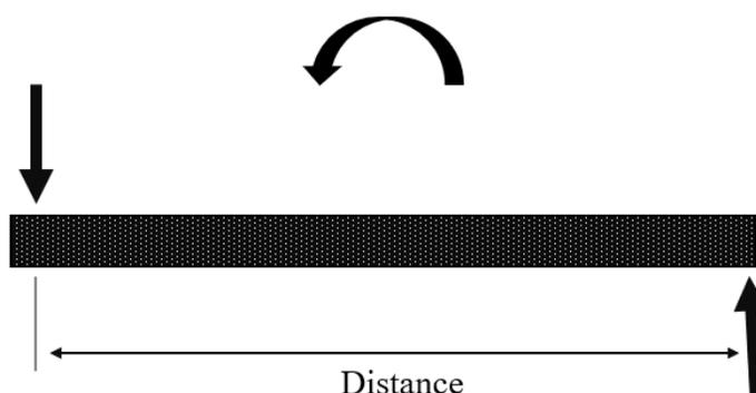
**Figure 4: A couple involves two non-collinear forces equal in magnitude but opposite in direction. The tendency of a couple to produce rotation is the Moment of a Couple and is equal to the magnitude of one of the forces multiplied by the perpendicular distance between the two forces**
