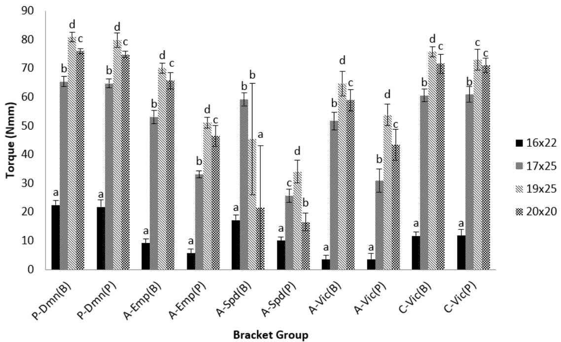
**Figure 29: Mean torquing moments in Nmm ( $\pm$ SD) measured at 45 degrees with different wire sizes (mil) versus bracket system. Error bars represent 1 SD, and letters shared within each bracket system cluster represent non-significant differences between wires at  $P > 0.05$**
