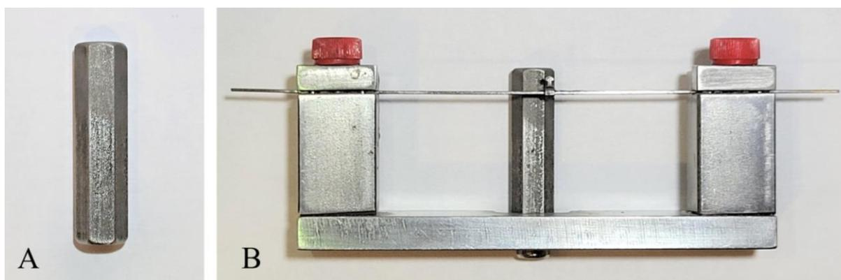
**Figure 14: Prepared hexagonal transfer pin (A), and assembled mounting jig including a 21.5 x 28 mil SS wire with crimpable stop and installed hexagonal transfer pin (B)**
