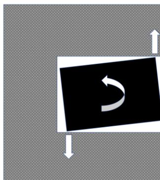
**Figure 8: Pictorial representation of a cross-section of wire twisting within a bracket slot to produce torque, as viewed from a mesial or distal view. The grey patterned area represents the bracket, black represents a wire engaged in the slot, central white arrow represents direction of torsion of the wire, and the vertical white arrows represent contact points of the wire against the slot walls, producing a couple that would generate torque**
