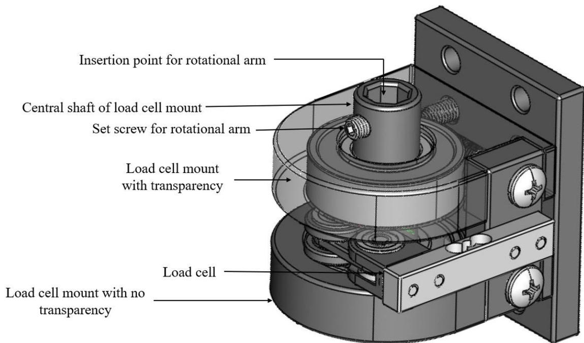
**Figure 17: Isometric CAD views of the load-cell mount and load cell with transparency added to highlight the innerworkings of this component. Labels highlight some of the various components of the torque-measuring fixture**
