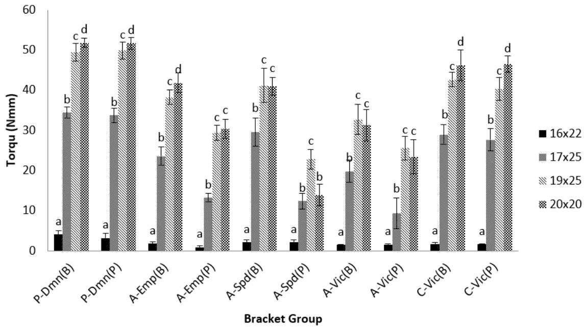
**Figure 28: Mean torquing moments in Nmm ( $\pm$ SD) measured at 30 degrees with different wire sizes (mil) versus bracket system. Error bars represent 1 SD, and letters shared within each bracket system cluster represent non-significant differences between wires at  $P>0.05$**
