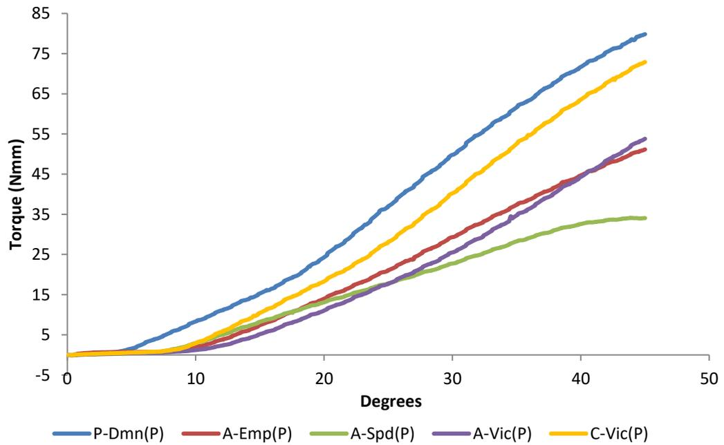
**Figure 22: Mean torquing moments measured for each bracket system and 19 x 25 mil SS wires, simulating both buccal (A) and palatal root torque (B)**
