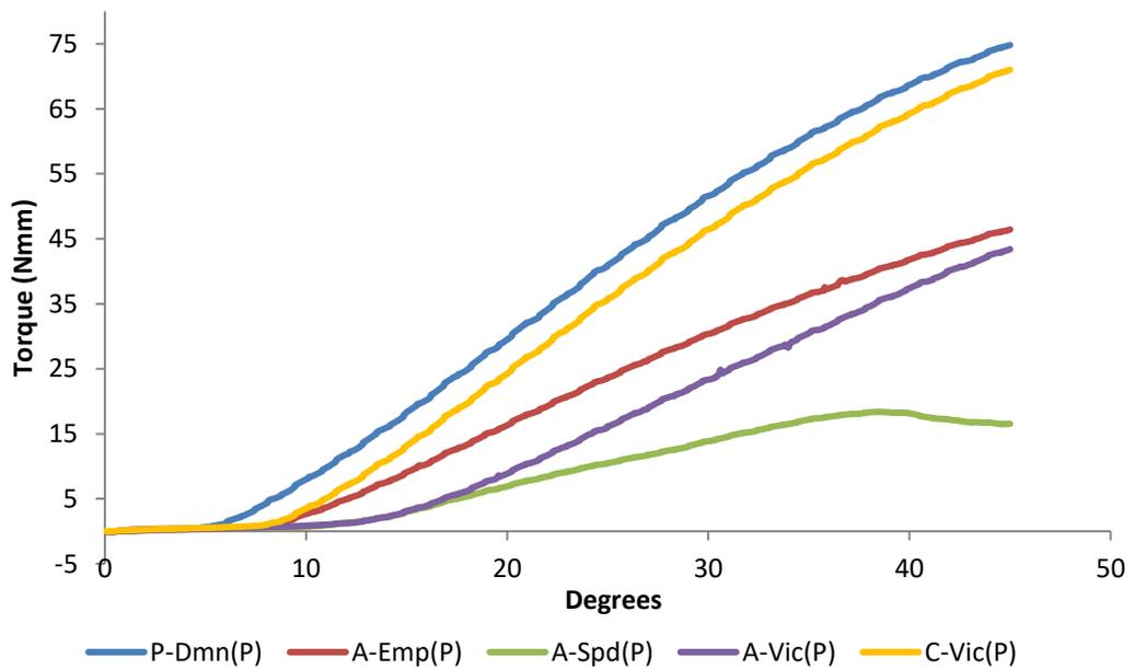
**Figure 23: Mean torquing moments measured for each bracket system and 20 x 20 mil SS wires, simulating both buccal (A) and palatal root torque (B)**
