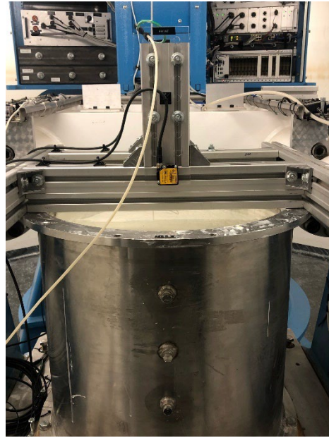
Figure 6-6 Solid tub used to prepare clay samples showing newly casted clay before spinning
