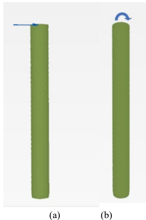
Figure 4-4 Procedure for stiffnesses determination for a monopile with 80m depth (a) for determining K_L and K_{LR} (b) for determining K_{LR} and K_R
