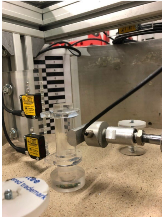
Figure 6-8 Side view of HF1 showing laser sensors used and load cell and actuator
