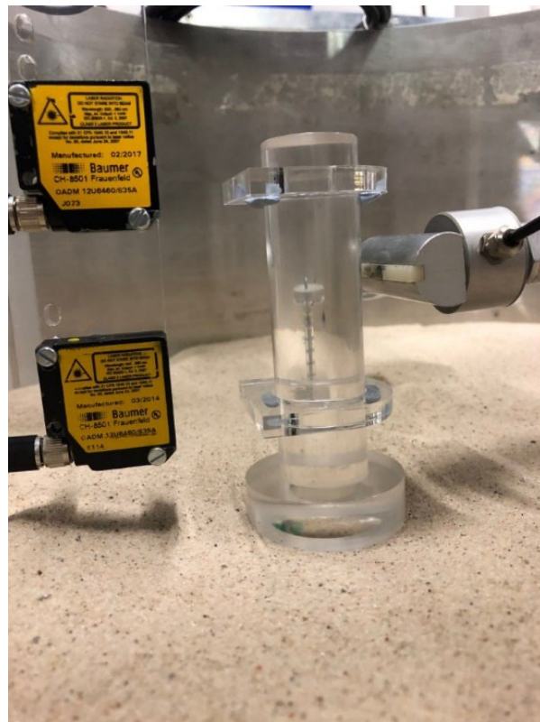
Figure 7-8 close up image showing pneumatic actuator and hybrid foundation with laser sensors
