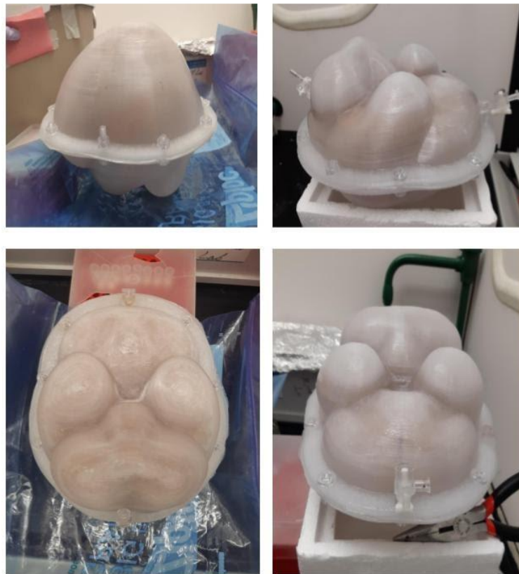
Figure 5. The brain shaped 3D printed container holding an ex vivo human brain.
