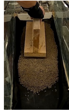
(c) Compaction of the top layer
