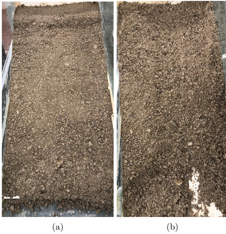
Figure 4.1: (a) Subgrade (sand) before the test was conducted and (b) after the failure
