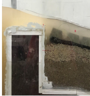
(b) Loss of contact on the upstream
