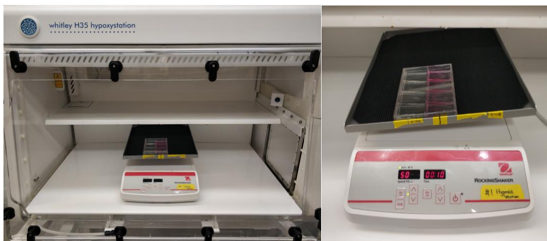
Figure 2.1 Rocking bioreactor system setup. Left: The rocking bioreactor system placed in the HypOxystation H35 system. Right: The operating rocking bioreactor system under the 11° 50 rpm rocking condition. The placement of the culture plate ensured that the centre of the wells in use were aligned with the rotating axis of the rocker.
