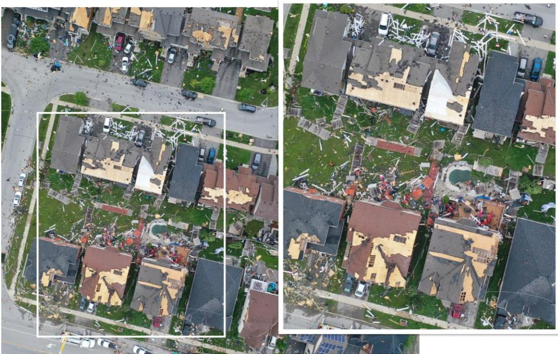
**Figure 8: Drone imagery of roof sheathing failures from Barrie tornado on July 15th, 2021, photo courtesy of Northern Tornadoes Project**
