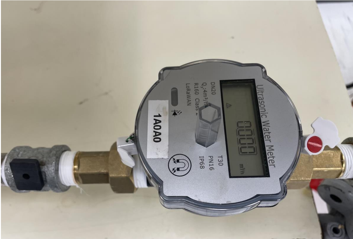
Figure 3.4 In-line ultrasonic flowmeter used in the experimental setup
