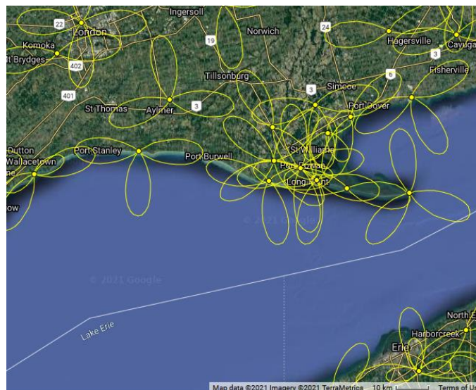
Figure 6: Motus towers (dots) and estimated antenna ranges (loops) in the Motus Wildlife Tracking System surrounding the release site (Motus.org, 2021)
