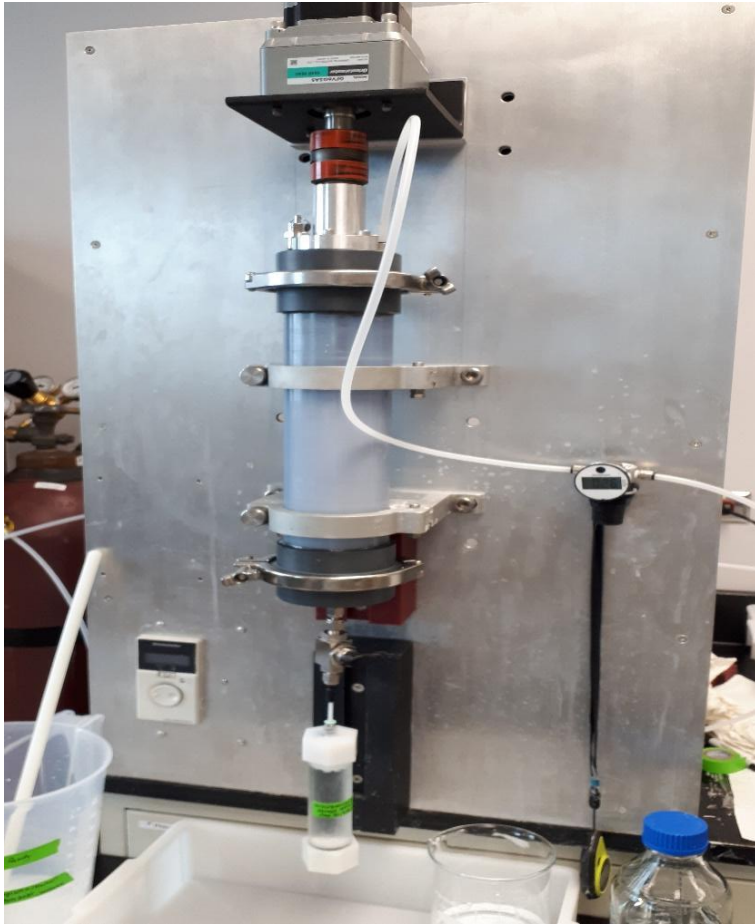
Fig 3.16: PPV with Column attached (as the column being packed)
