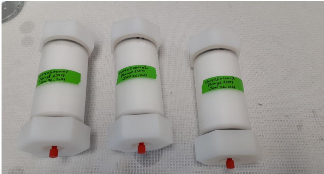
Fig 3.17: Columns Packed (Columns packed and ready for Analysis)
