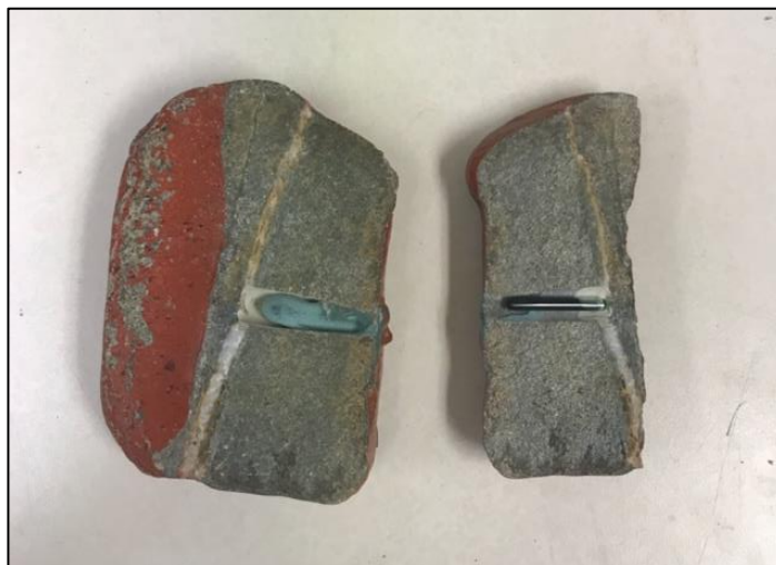
Figure 9. Example of a prepared 64-90 mm tracer stone, with 32 mm PIT tag (right).
