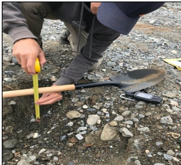
Figure 13. Measuring tracer burial depth from top of the bed surface (shovel handle) to the top of the tracer stone.
