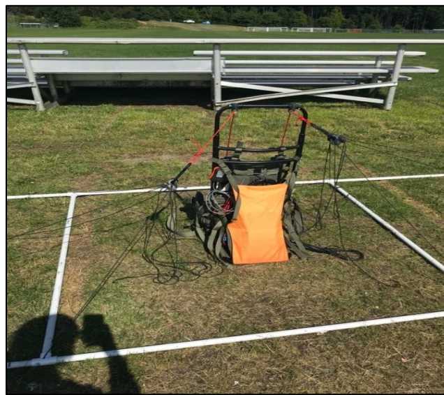
Figure 12. Large antenna cord system with backpack fastened to PVC pipe frame using ropes, pulleys, and cams.
