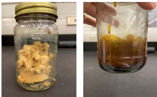
Figure 6 Left: wax product collected from oil fraction at lower temperatures. Right: liquid oil collected from the oil fraction at the higher temperatures.
