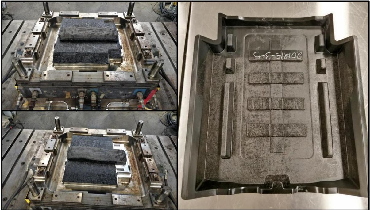
*Figure 17: LFT-D charge laid on top of GMT sheets for moulding in tailored sheet (top left) and rectangular sheet (bottom left) configurations alongside a finished part (right)*
