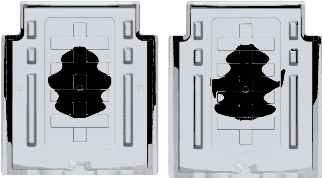
*Figure 20: A sample of two warpage patterns to be compared via SSIM*
