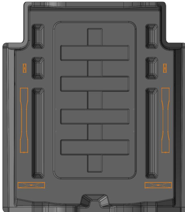
Figure 24: Mechanical testing sampling locations (top: short beam shear; middle: tensile; bottom: flexural)
