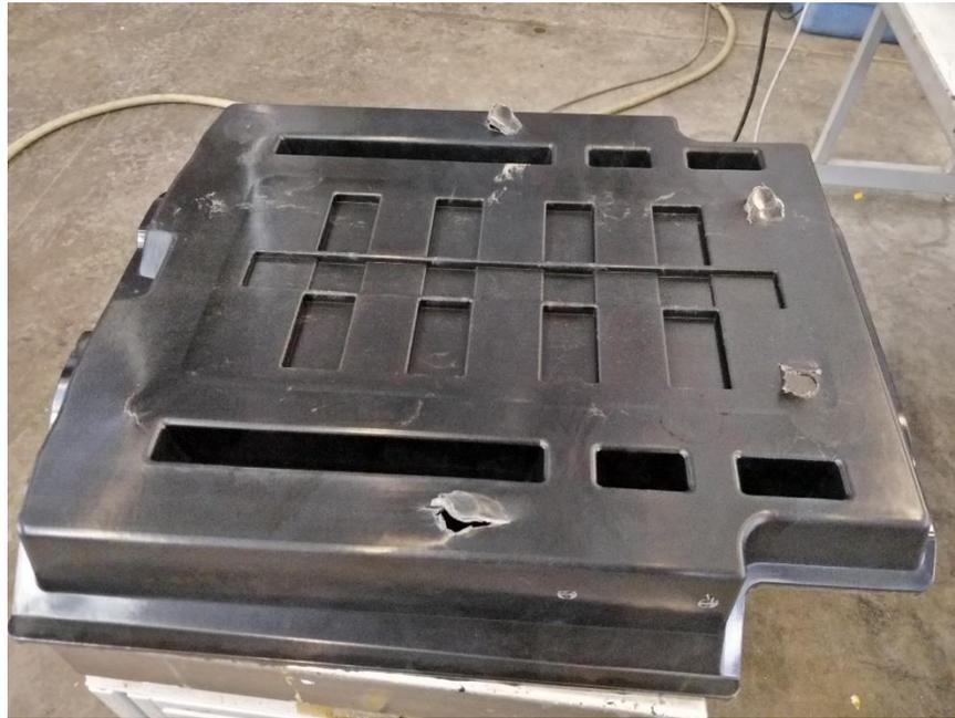
*Figure 18: Finished part destroyed by ejector pins*
