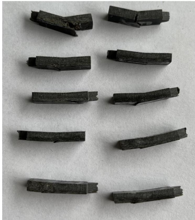
*Figure 26: Post-fracturing short beam shear specimens*
