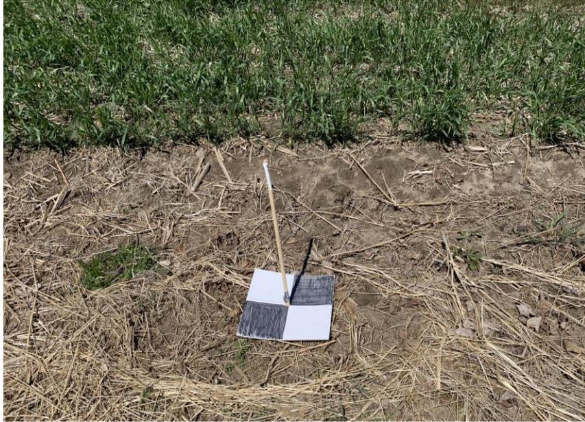
**Figure A 1. Example of ground control point marker.**
