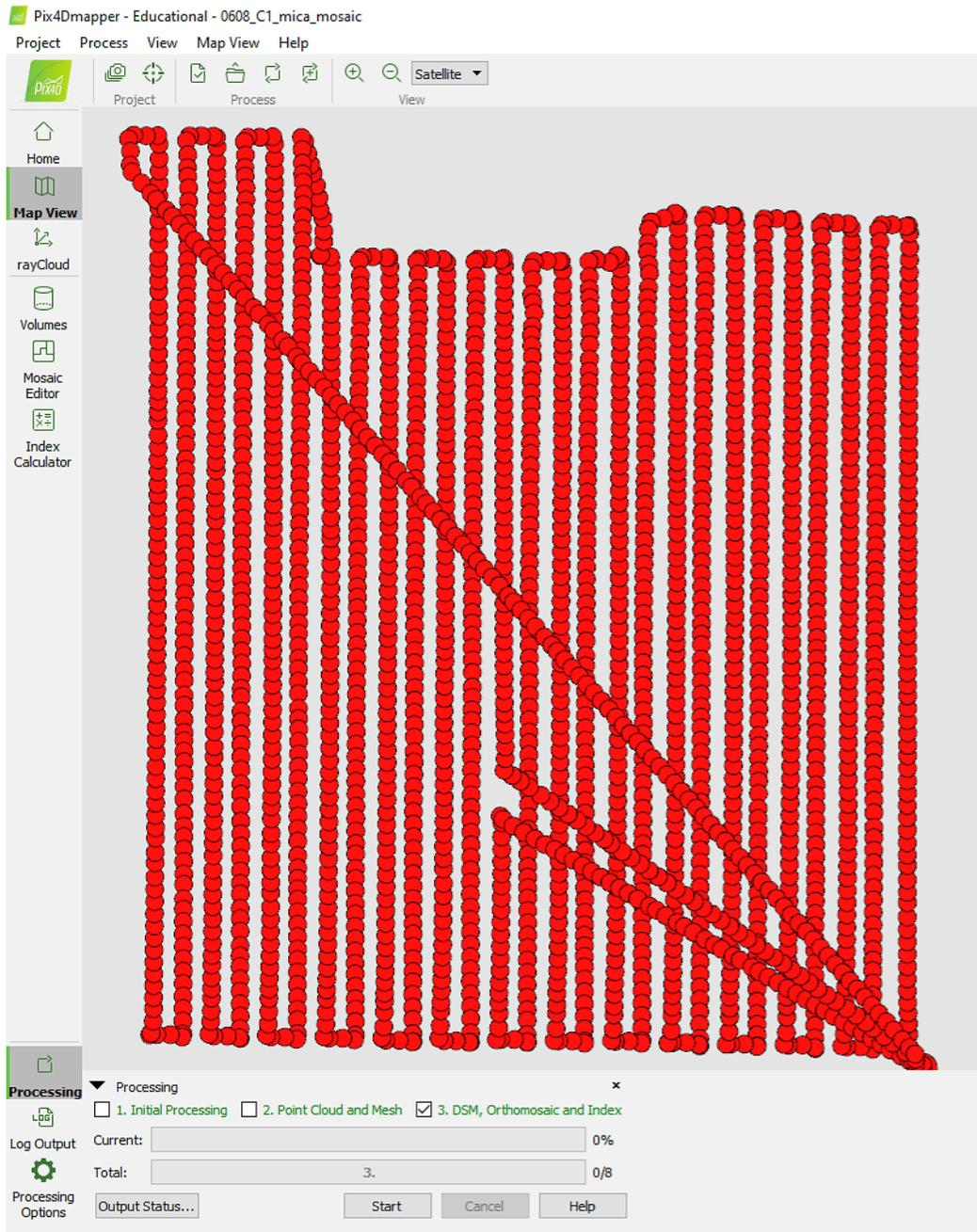
**Figure B 1.** Example of Pix4Dmapper flight pattern map view. Each red circle represents the UAV's location with the sensor taking a picture. The diagonal flight patterns are due to the UAV returning to the starting point for a battery change midway through and returning upon completion of the specified flight area.
