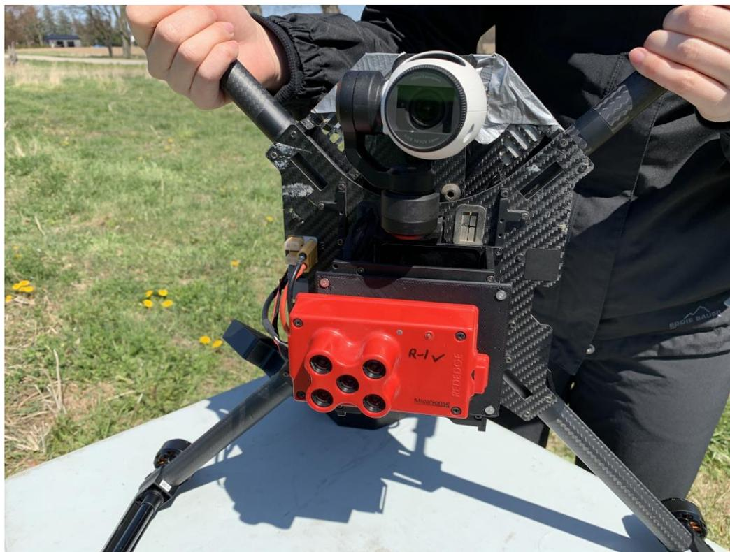
**Figure A 3. Sensors attached to the underbody of the DJI Matrice 100 UAV. The RGB camera is on the top, and the red MicaSense RedEdge camera with five sensor bands is on the bottom.**
