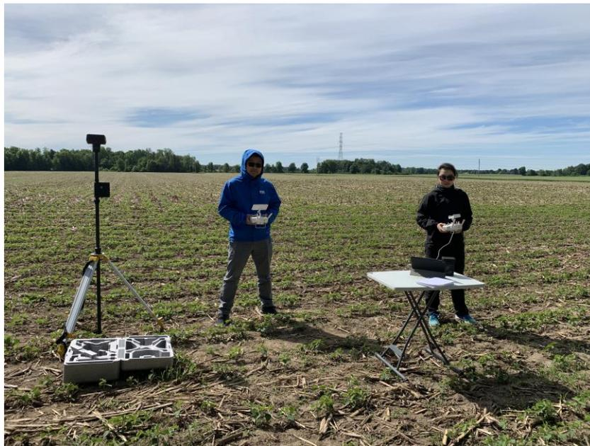
**Figure A 2. Piloting the unmanned aerial vehicles. The tall device on the left is the real time kinematic (RTK) navigation base station.**
