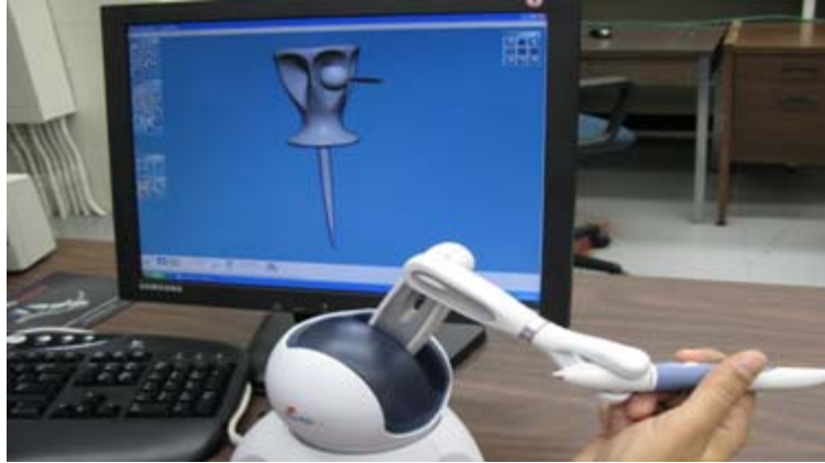
Figure 2.1 Haptic interaction with a virtual model through a haptic device (PHANTOM® Omni of SensAble Technologies, 2008) located at the University of Western Ontario.
