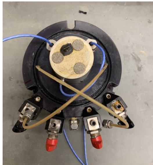
Figure 4.5: Compression crystals and bender elements installed on triaxial platen
