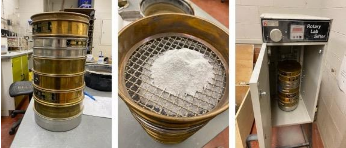
Figure 28. (Left) Assembled sieve stack; (Middle) Sample (UWO-1G pictured) added from the top (No. 4) sieve; (Right) Stack placed into a mechanical shaker to sift for 12 minutes.
