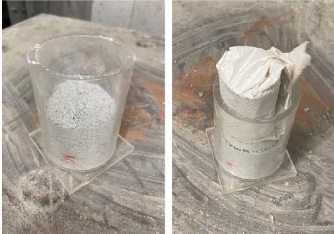
Figure 37. Sample (LHS-1 pictured) was added to half the mould's depth (left) and vibrated for natural compaction with a weight to stop any loss in quantity (right). This step was repeated until the mould was fully filled with compacted sample.
