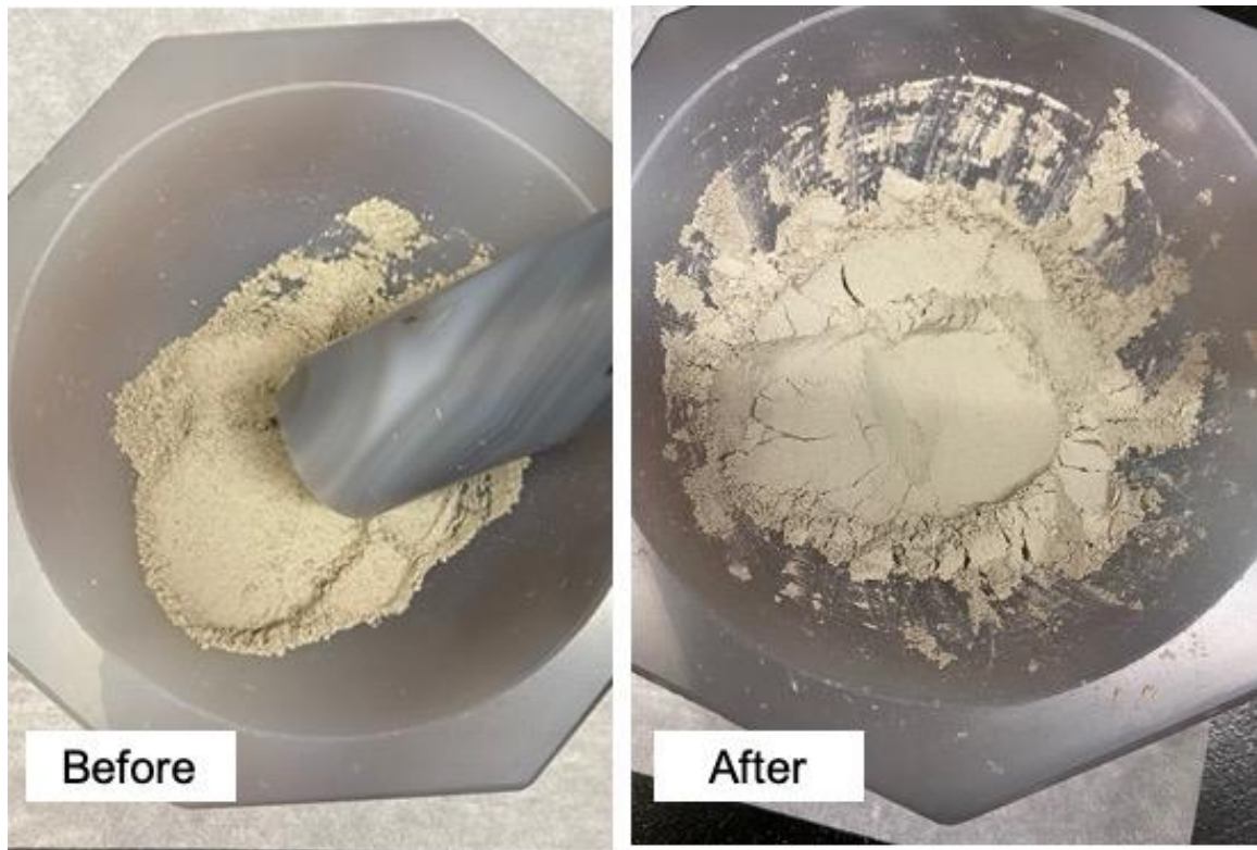
Figure 33. Sample grinding in preparation of XRD characterization. Sample shown in the figure is the Mistastin impact melt used to produce UWO-1S.
