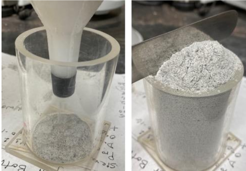
Figure 36. Sample (LHS-1 pictured) is loosely sprinkled into the mould through a funnel (left) and flattened with a spatula at the top (right).
