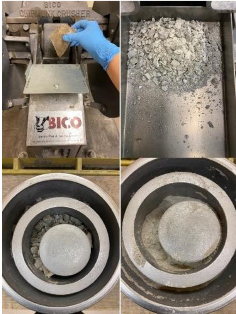
Figure 23. Rocks (impact melt rocks pictured) were tossed into the Bico crusher (upper left) and crushed into smaller masses (upper right), then transferred into the ring pulverizer container (lower left) to be ground into powder-like product (lower right).
