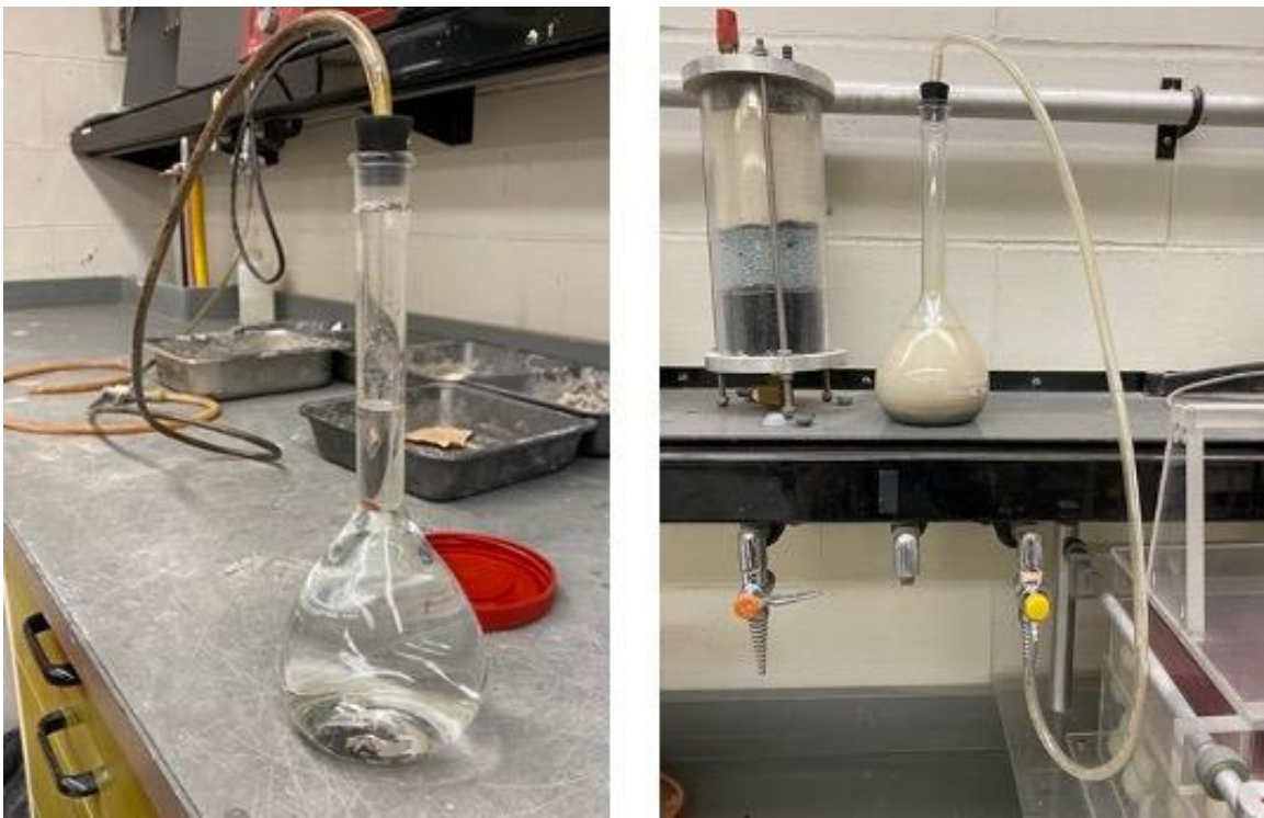
Figure 35. (Left) De-airing 500ml distilled water in a volumetric flask; (Right) De-airing sample mixture (LHS-1 pictured) for 24h.
