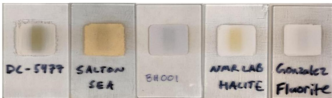
**Fig. 6-2: X-ray burn on a selection of samples after pXRD analysis. From left to right: DC-5477, Salton Sea, DeLaval Blue, 99.9% AnalR, Gonzales Fluorite.**
