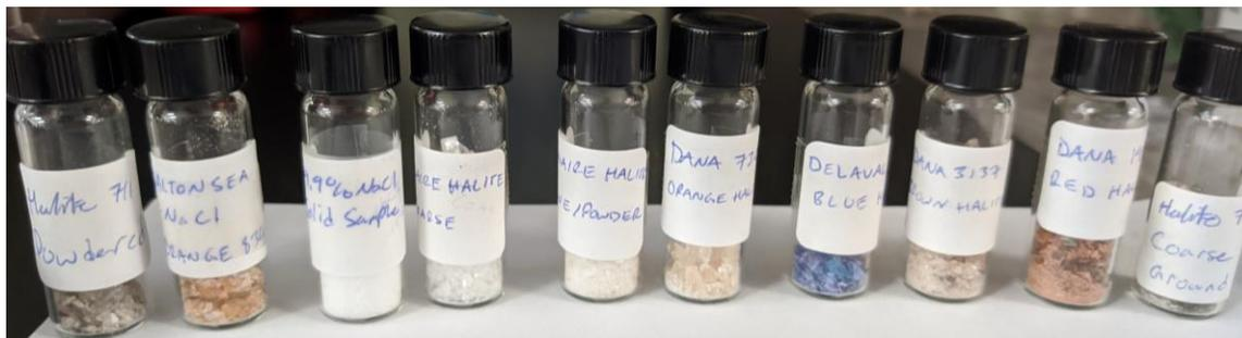
**Fig. 2-3: Coarsely ground halite samples prepared for NMR analysis.**
