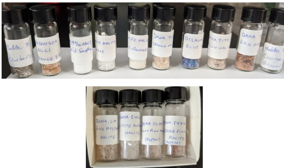
**Fig. 3-4: Coarsely ground halite samples for NMR analysis. Samples are as follows: Top: DC-711 Powdered, Salton Sea, 99.9% Reagent grade halite, coarsely ground Bonaire, fine grained Bonaire, DC-730, DeLaval Blue, DC-3137, DC-1922, and DC-711 coarsely ground. Bottom: TronaCA, DC-5490, DC-5477 (light pink), and DC-5477 (dark pink).**
