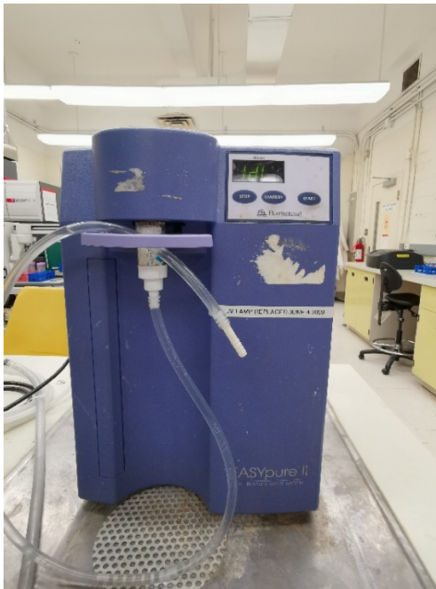
Figure 4-3: Water purification system.
