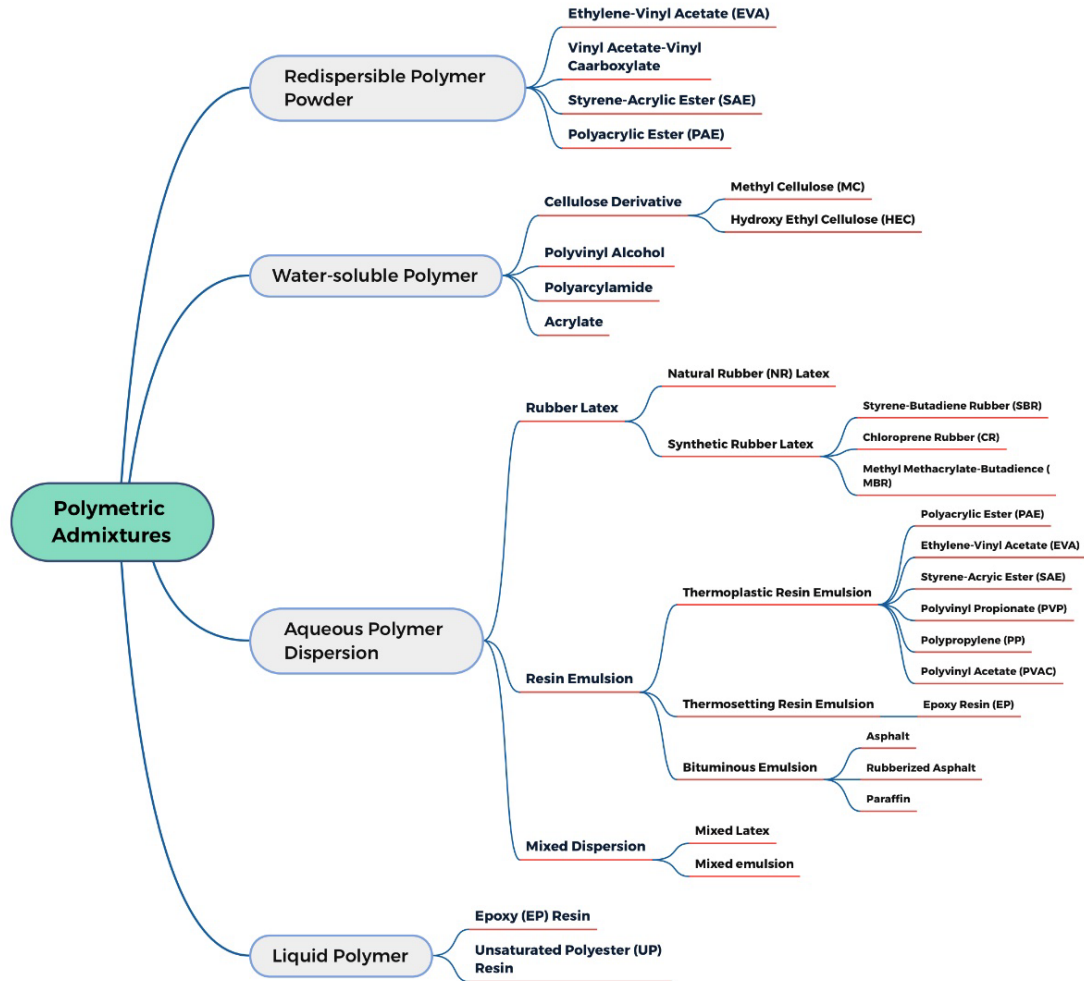
Figure 2-3: Classification of polymeric admixtures for PMC. Reproduced from (Ohama, 1997).
