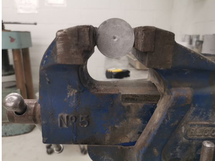
Figure 4-2: Cracking specimens using a screw jack.
