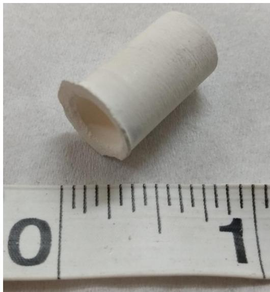
**Figure A 5: Zirconia cylinder before turning on a lathe, with inch scale**
