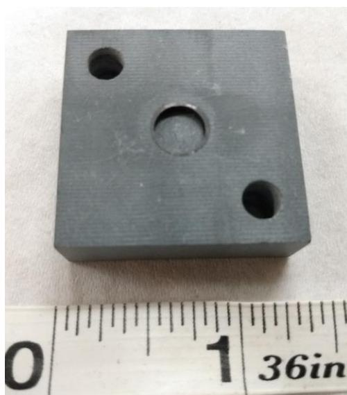
**Figure A 4: The reverse side of the slab in Figure A 3 with recessed space where zirconia disk will be emplaced for thermally insulating sample**
