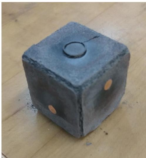
**Figure A 8: A post-experimental cubic pressure cell, edge length of ~25 mm**
