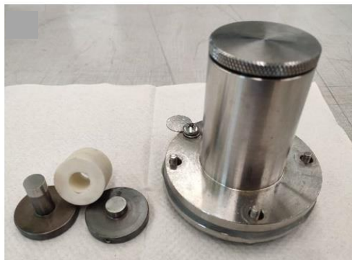
Figure 3.11 A real photo showing the mold cell with the internal parts and the shell.
