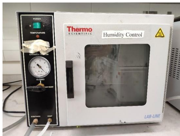
Figure 3.10 The customized humidity-control chamber based on a vacuum oven. A hygrometer is placed in the chamber to indicate the real-time humidity value.
