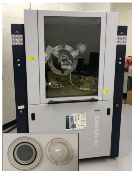
Figure 3.6 The Bruker D8 Advance Diffractometer XRD system. The inset show the holder that prevent the air-sensitive samples (e.g., SSEs, electrode) from air exposure.
