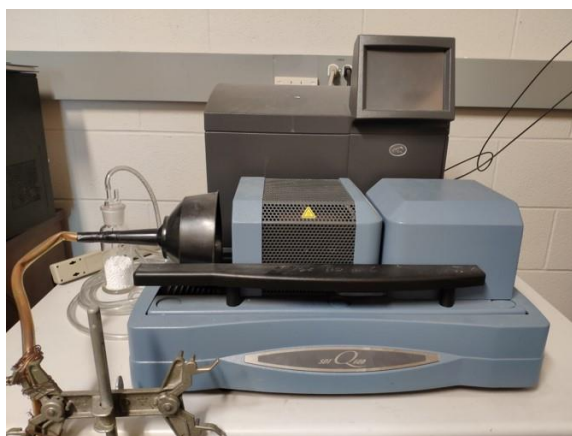
Figure 3.8 The SDT Q600 by TA Company to carry out the TGA-DSC measurements
