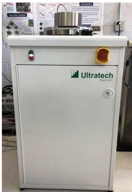
Figure 3.3 The Savannah 200 ALD system produced by Veeco Instruments Inc. in the USA.
