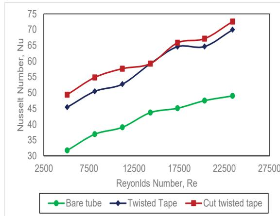
**FIGURE 3.** Comparison of Nusselt number at various Reynolds number for bare tube, twisted tape and cut twisted tape inserts
