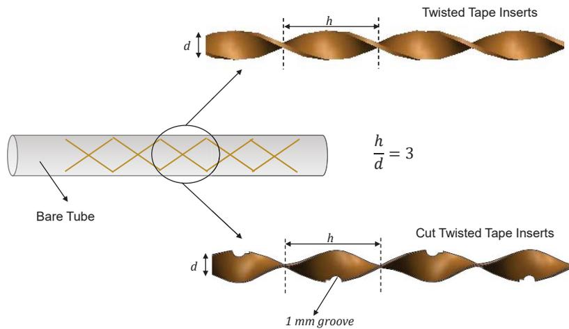
FIGURE 2. Representation of inserts used within the bare tube – twisted tape and cut twisted tape
