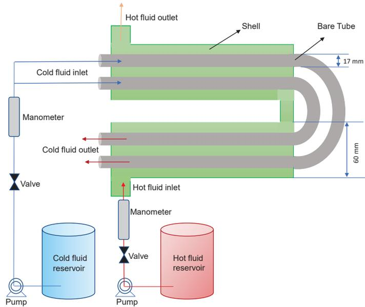
FIGURE 1. Experimental setup of the double pipe heat exchanger
