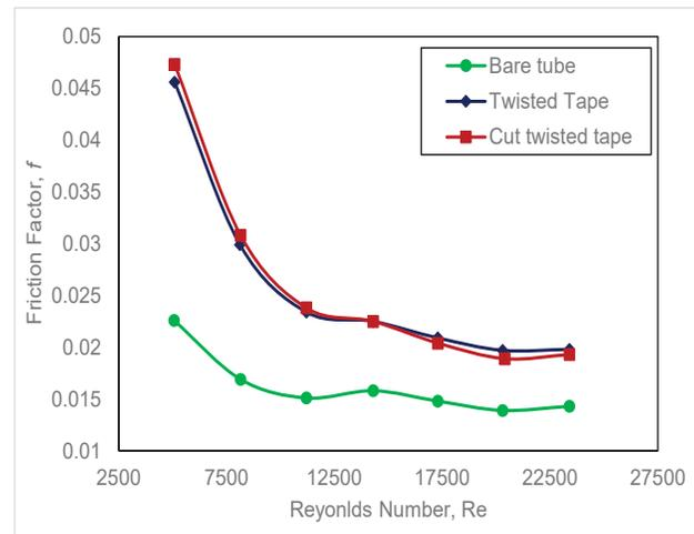
**FIGURE 5.** Comparison of friction factor at various Reynolds number for bare tube, twisted tape and cut twisted tape inserts
