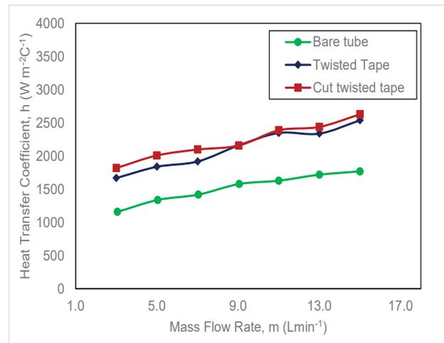
**FIGURE 4.** Comparison of heat transfer coefficient at various Reynolds number for bare tube, twisted tape and cut twisted tape inserts
