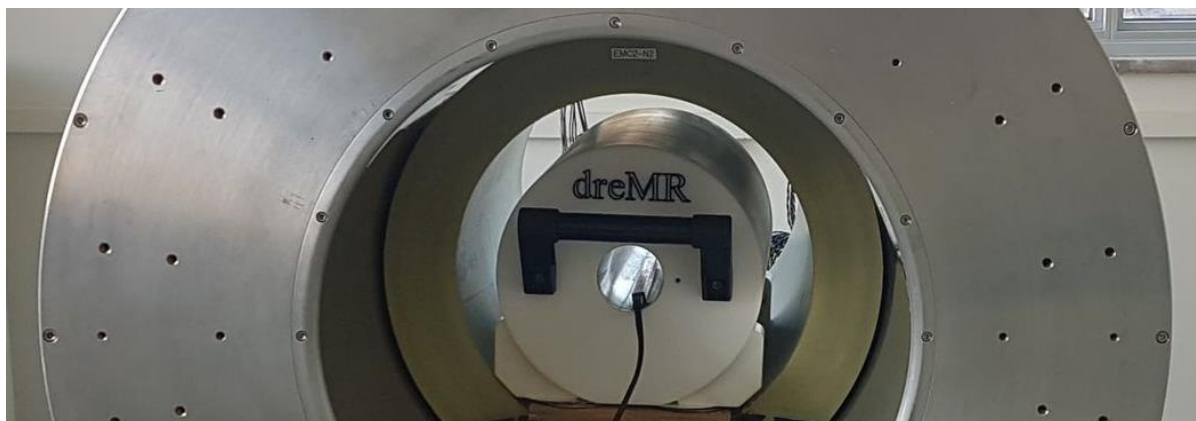
Figure 4.2. The dreMR insert coil (white) placed within our 0.5T cryogen-free superconducting magnet, so that their isocenters coincide. A gradient coil (green) is present but was not used during this experiment.
