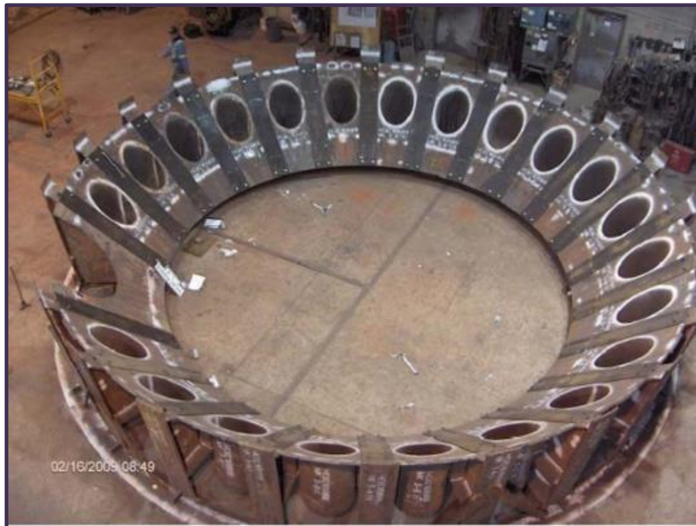
Figure 1.3 Ring baffle with flux-tube in a Coker [15]
