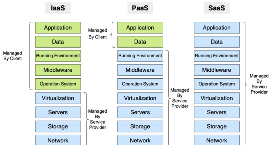
**Figure 2: Cloud Service Type and Layers**
