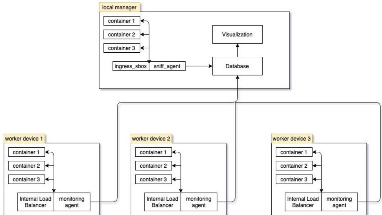
**Figure 9: System Architecture**
