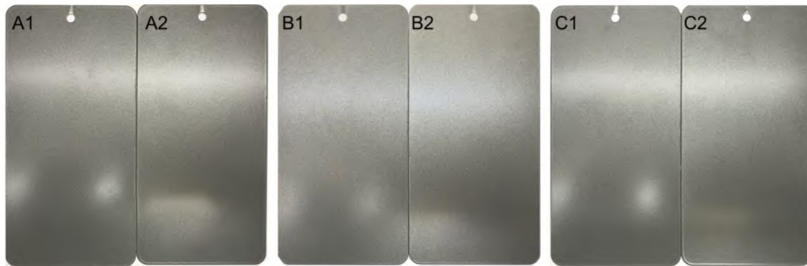
Figure 8.9: The images of films prepared at 1 and 3 bar from different powders. A) non-bonded; B) commercial bonded; C) microwave bonded.
