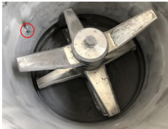
Figure 8.4: The four-layer agitator inside the bonding tank.
