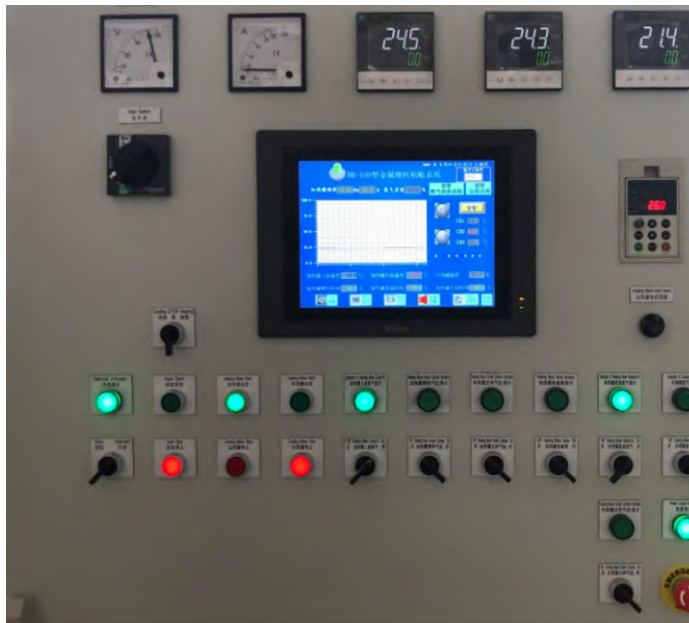
Figure 8.5: The control panel of the industrial microwave bonding machine.
