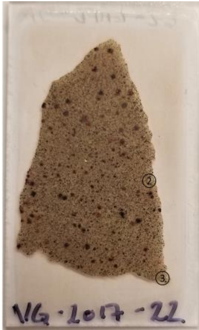
Figure B-19. VG-2017-22 thin section showing spots analyzed
