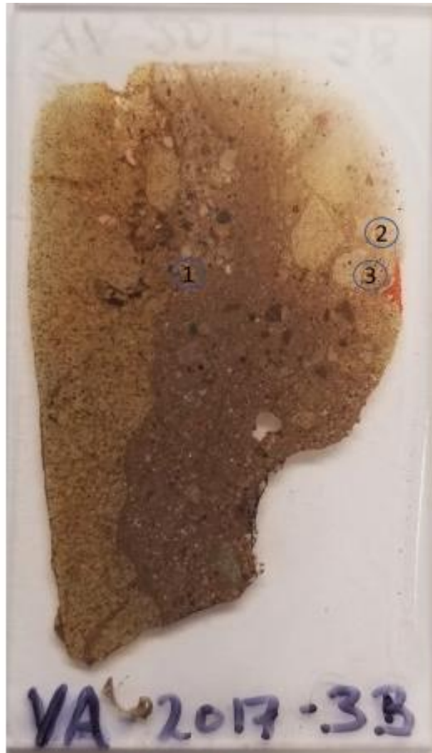
Figure B-8. VA-2017-3B thin section showing spots analyzed
