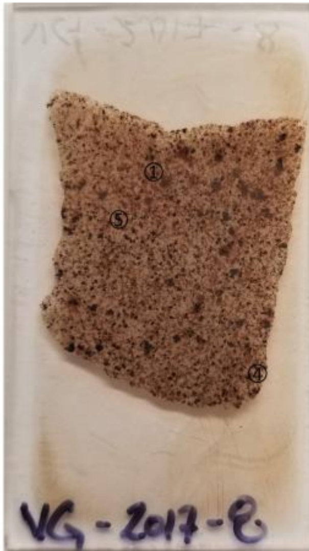
Figure B-12. VG-2017-8 thin section showing spots analyzed
