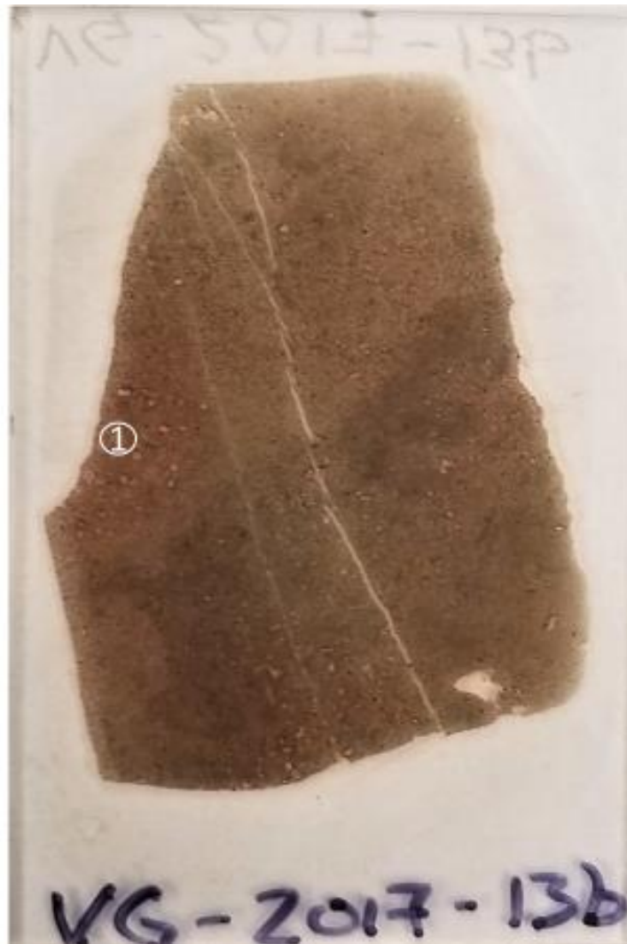
Figure B-16. VG-2017-13B thin section showing spots analyzed
