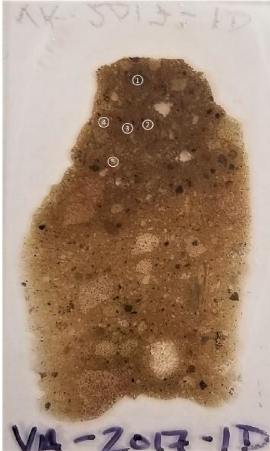
Figure C-3. VA-2017-1D thin section showing spots analyzed
