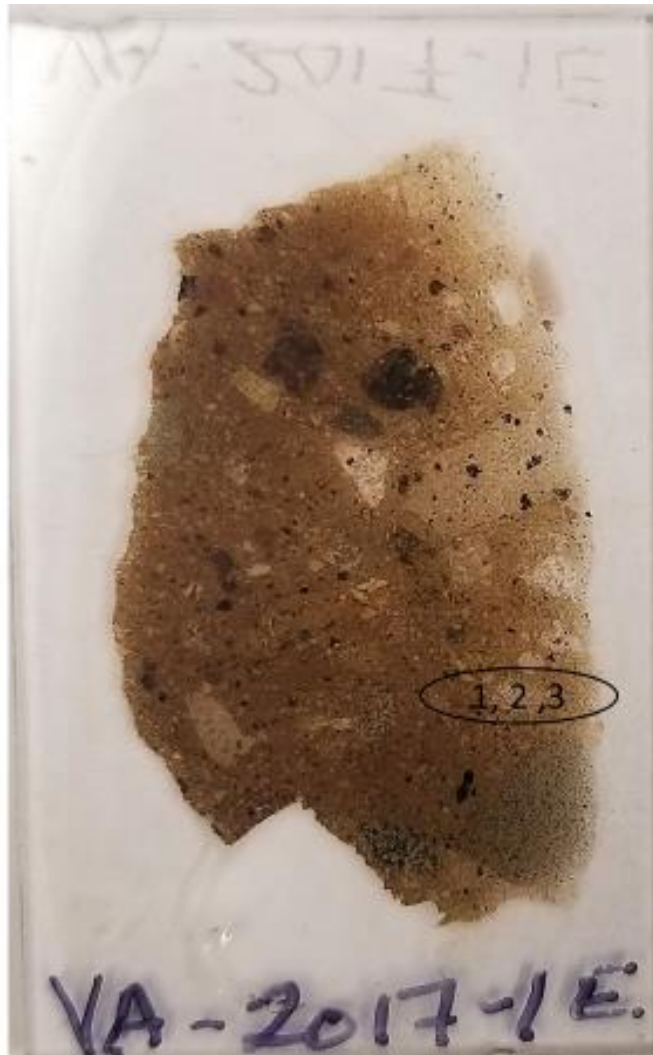
Figure B-4. VA-2017-1E thin section showing spots analyzed
