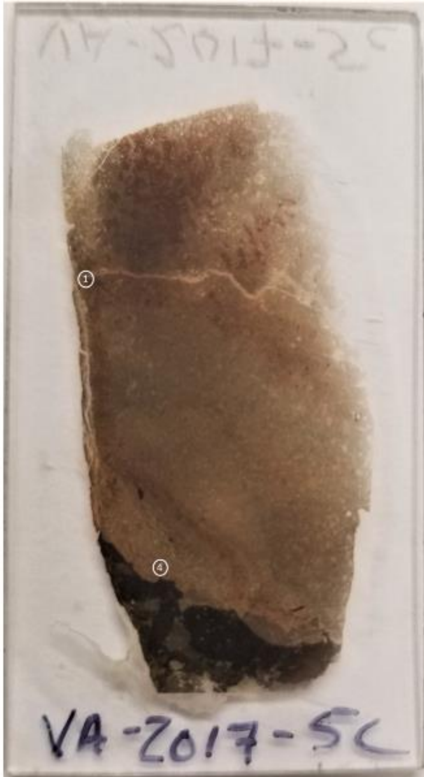
Figure C-4. VA-2017-5C thin section showing spots analyzed
