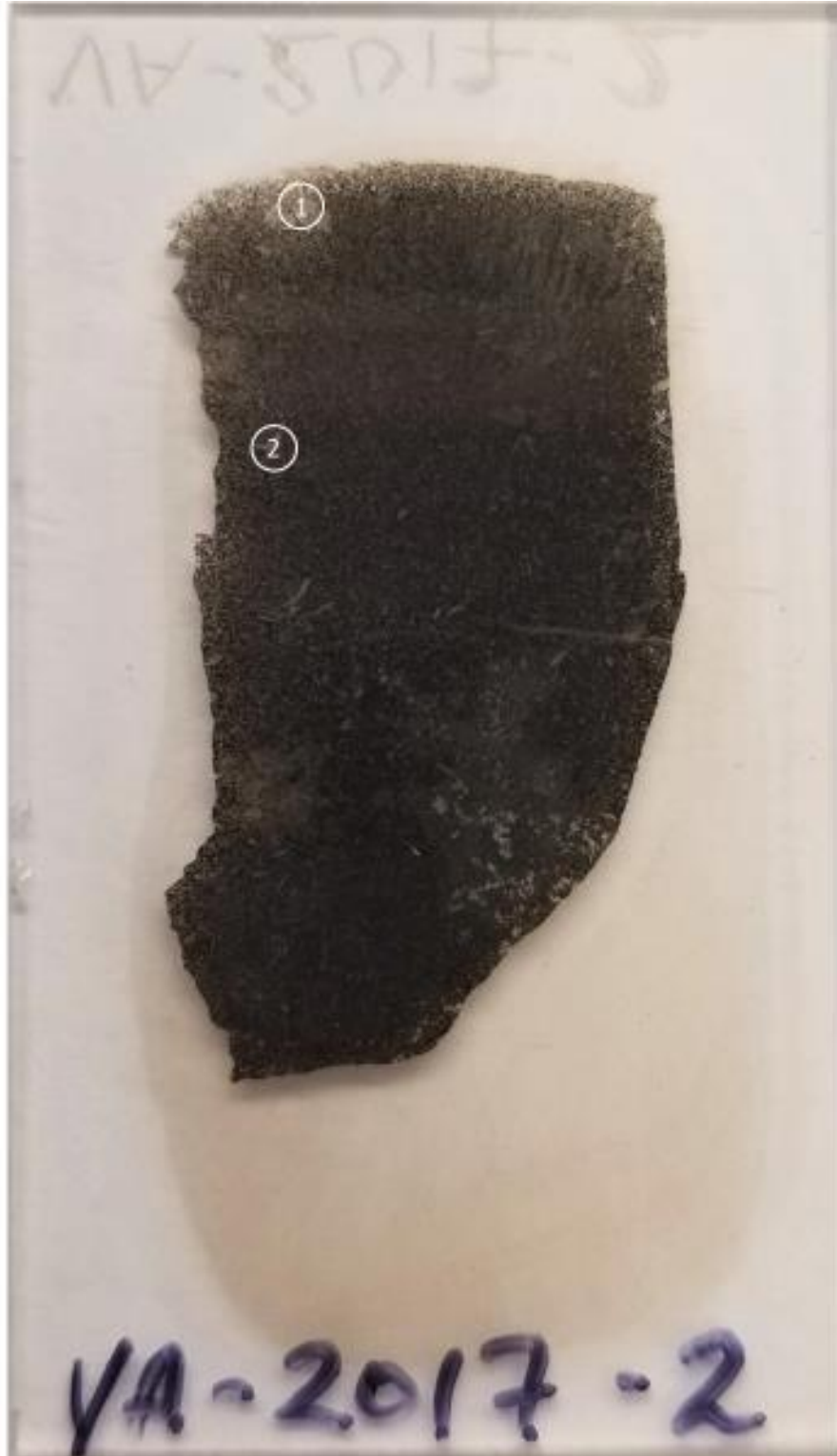
Figure C-5. VA-2017-2 thin section showing spots analyzed
