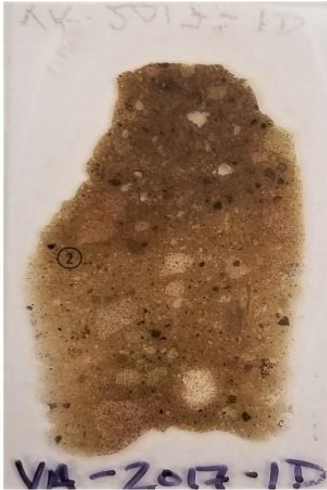
Figure B-3. VA-2017-1D thin section showing spots analyzed
