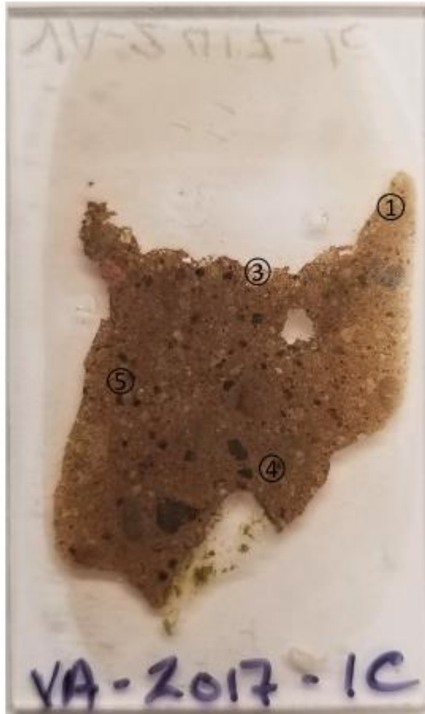
Figure B-2. VA-2017-1C thin section showing spots analyzed
