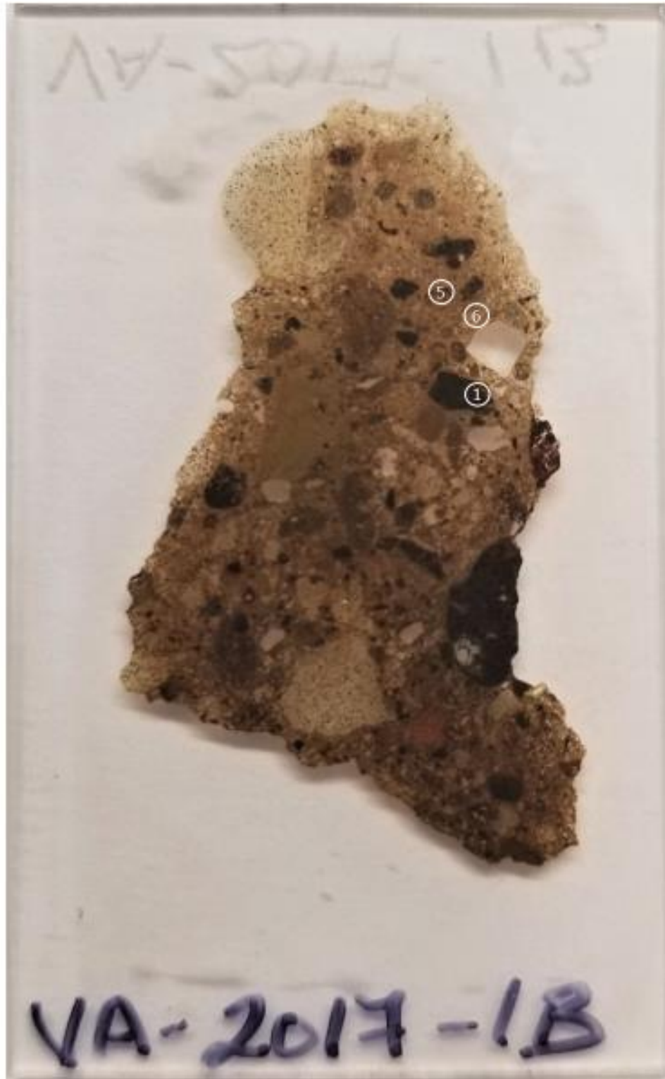
Figure C-2. VA-2017-1B thin section showing spots analyzed
