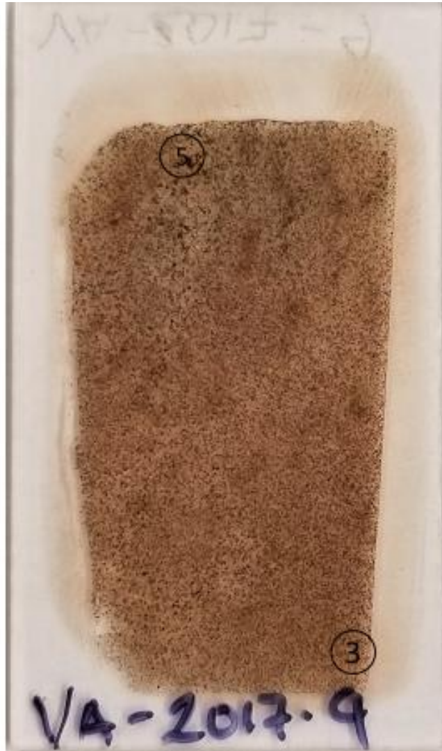
Figure B-13. VG-2017-9 thin section showing spots analyzed
