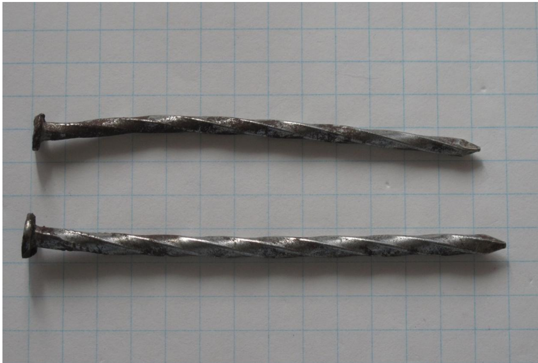
Figure 2.2 Photograph of the two types of nails used for the toe-nail RTWC on the test House. The grid shown is 6mm by 6mm, above is the 12d nail, below is the 16d nail.
