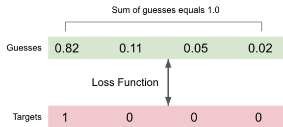
Figure 19: A visualization of guess and target vectors being compared. The sum of all guess probabilities must equal 1.
