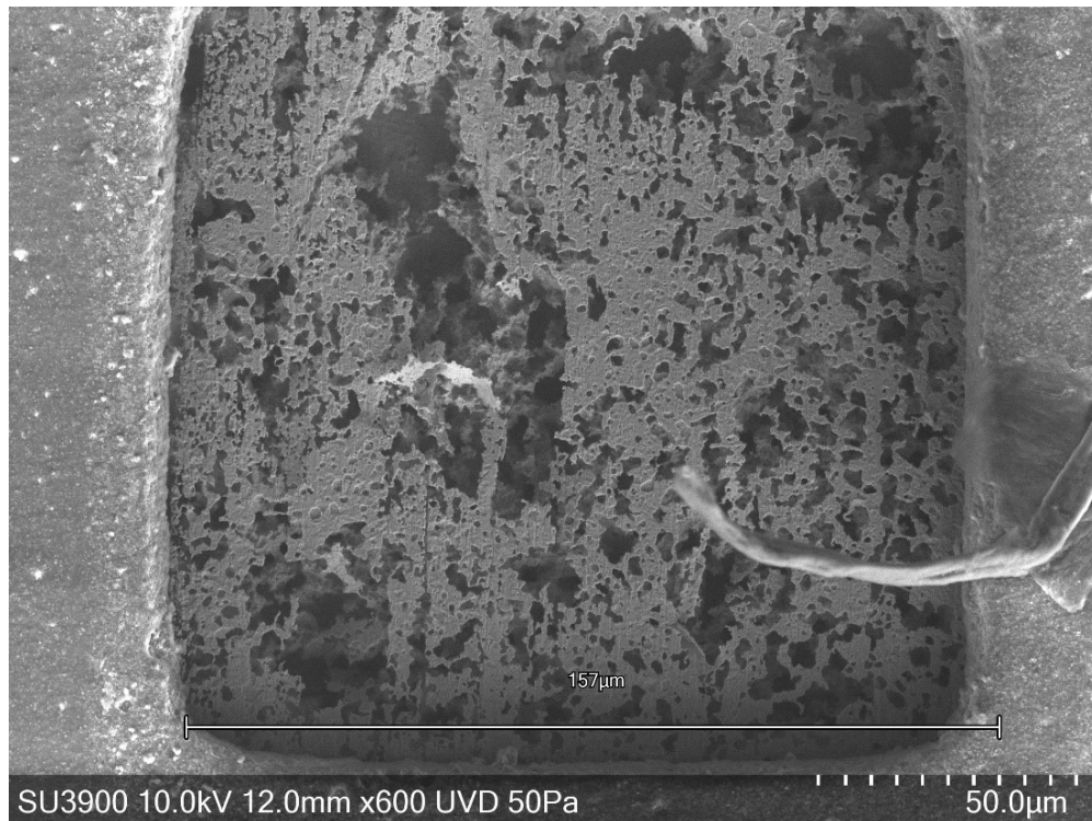
Figure 6.31. A SEM image of electrode 1,3 on CB0E after 8 hours of immersion in the Ar-sparged pH 1.5, 0.0374 M [Cu] potential buffer
