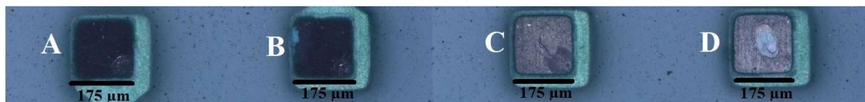
Figure 6.44. Optical images of electrodes 3,3-3,6 after 1 day of immersion in 10^{-3} M \text{SH}^- , highlighting the difference in film grown between the pre-grown \text{Cu}_2\text{S} films and the previously clean Cu
