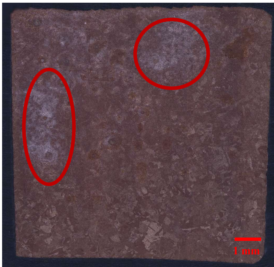
Figure 4.5. An optical image of a Cu coupon surface after applying CC = 1000 \mu\text{A} in 1 M NaCl in the anaerobic chamber. Spots showing an unidentified white film are circled in red
