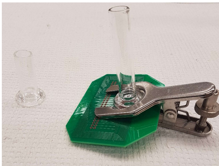
Figure 1.10. The assembled microcell clamped onto an array sealed with an O-ring and the pressure applied by the clamp. An additional smaller cell can be seen to the left
