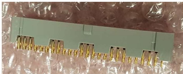
Figure 3.1. A profile view of a blank rectangular 50 pin male header
