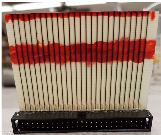
Figure 3.8. A second generation MEA coated with Microshield to limit the amount of Cu exposed to solution
