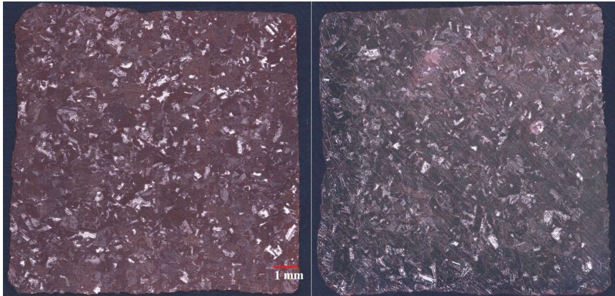
Figure 4.10. Optical images of the entire Cu coupon surface after applying CC = 250 \mu A in 1 M NaCl in the anaerobic chamber (left) and on the benchtop (right)
