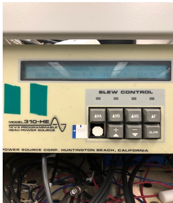
Figure 8.16: AC voltage source.
