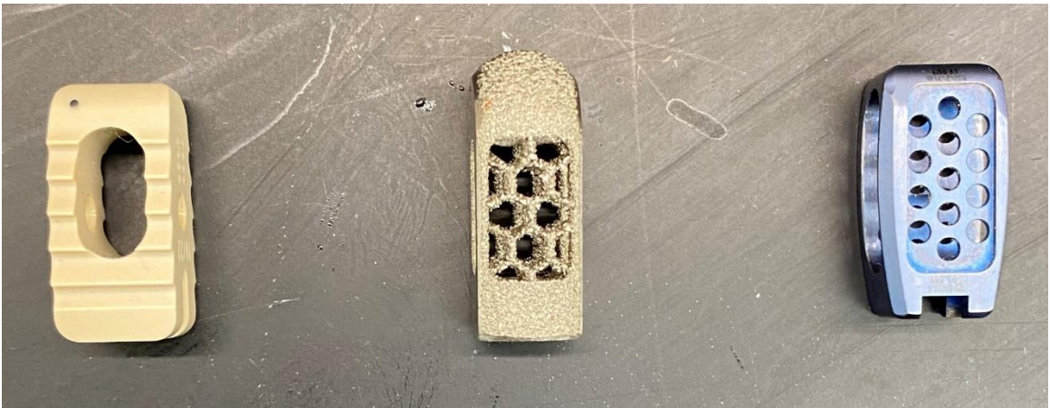
Figure 3. The picture shows 3 different types of cages. The first on the left, made of PEEK, the other two are made of titanium.
