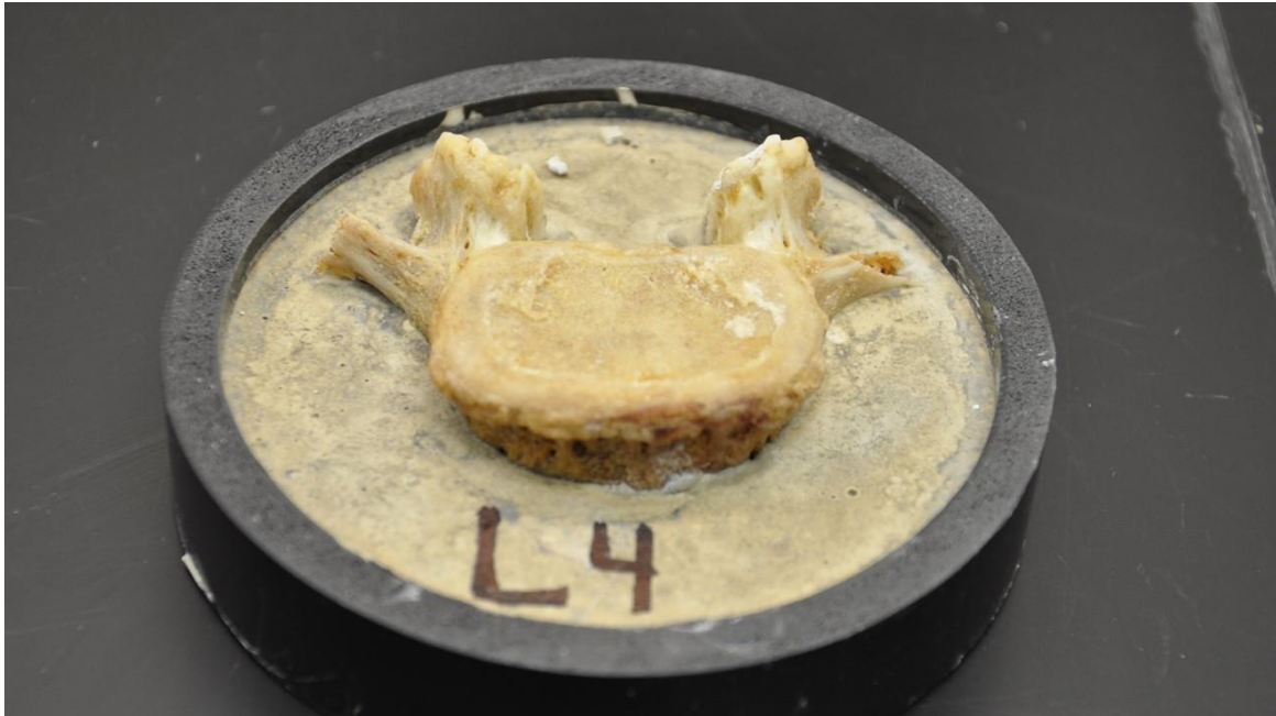
Figure 13. L4 vertebra potted in cement for biomechanical testing.
