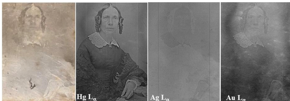
Fig. 2. A 19th century daguerreotype of the portrait of a lady from the collection of NGC in Ottawa. From left to right, the photo of the plate, the Hg L_{\alpha} XRF map, the Ag L_{\alpha} and the Au L_{\alpha} XRF map recorded at the 20 ID beamline of the APS using a 50 \mu\text{m} \times 50 \mu\text{m} beam at 13.5 keV, with 50 \mu\text{m} steps and 200 ms integration time.
