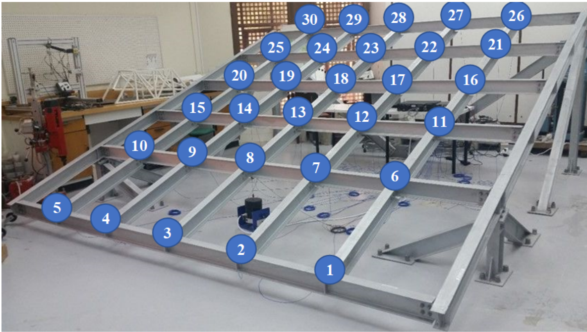
Figure 6.4: QUGS testbed, where the joints are numbered from 1 to 30 [4].
