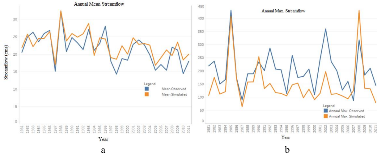
Figure 3- 17: Annual mean (a) and max (b) of observed and simulated streamflow values for 30 years from 1981 to 2011.
