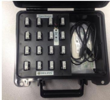
Figure 3.1: The Trigno wireless myoelectric system
