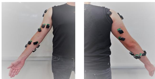
Figure 3.2: Trigno EMG sensors attached to the muscles of interest
