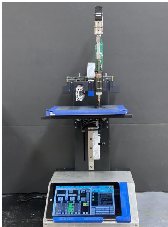
Figure 2-1 A picture of Engine SR 3D printer with KR2 15 modular printing heads from Hyrel 3D.
