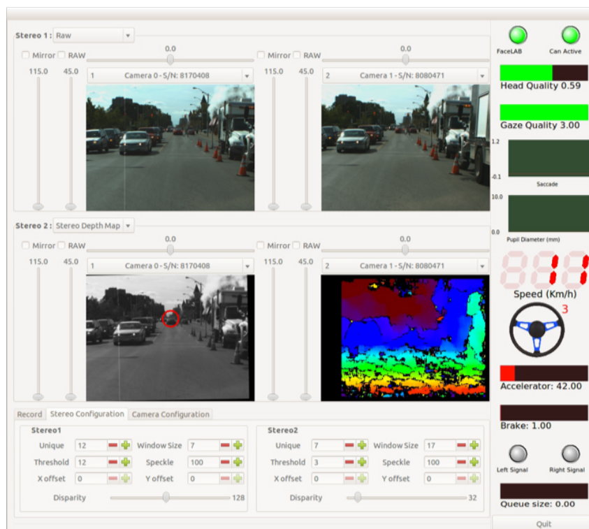
Figure 2.3: The on-board data recorder interface displaying depth maps, driver PoG, vehicular dynamics, and eye tracker data.
