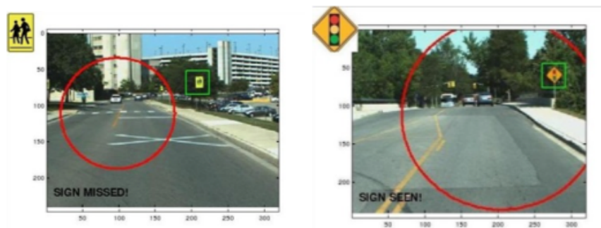
Figure 2.5: Two projections of the visual attention cone base on the stereo imaging plane.
