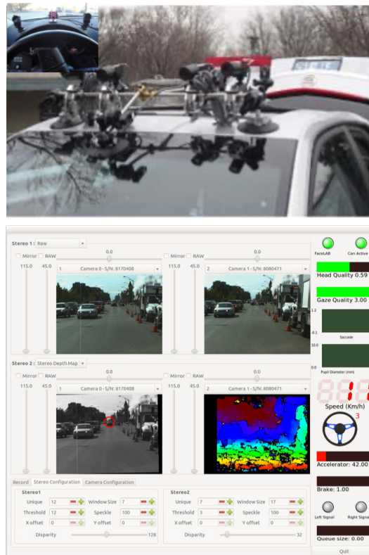
Figure 5.1: RoadLAB configuration. (top) : vehicular configuration: stereoscopic vision system on rooftop and 3D infrared eye-tracker located on the dashboard. (bottom) : software systems: The on-board system displays frame sequences with depth maps, dynamic vehicle features, and eye-tracker data.
