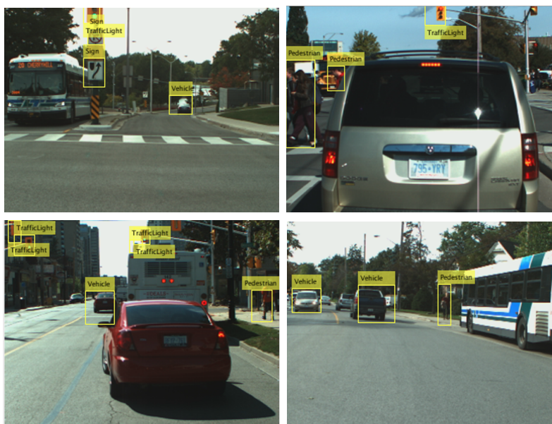
Figure 3.7: Examples of model A missing large vehicle objects.
