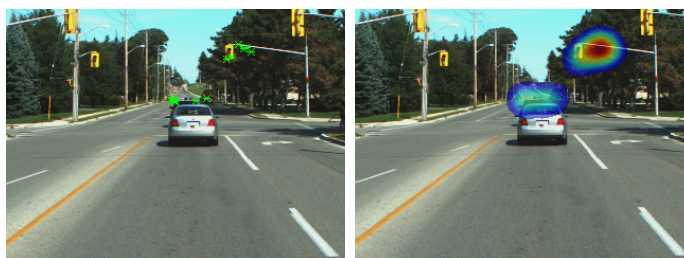
Figure 5.2: An example of PoG and matching fixation saliency map. (left): PoGs projected onto the forward stereo system of the vehicle obtained with the preceding 15 consecutive frames. (right): The driver's point of gaze as a 2-D Gaussian distribution.
