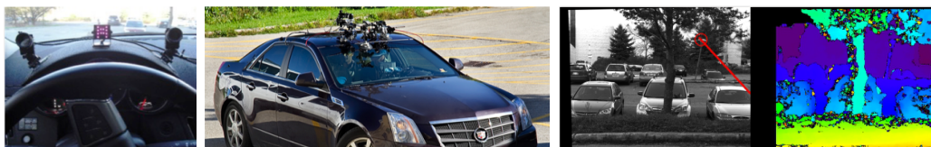
Figure 2.1: a) (left): 3D infrared gaze tracker; b) (center): Forward stereoscopic vision system on rooftop; c) (right): Driver PoG and LoG expressed in the reference frame of stereoscopic vision system and corresponding depth map.
