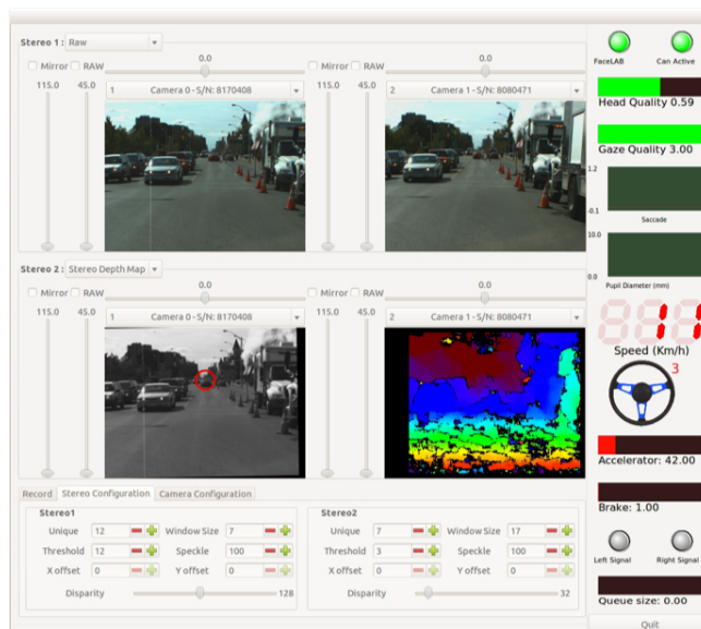
Figure 6.3: RoadLab software systems: The on-board system displays frame sequences with depth maps, dynamic vehicle features, and eye-tracker data.
