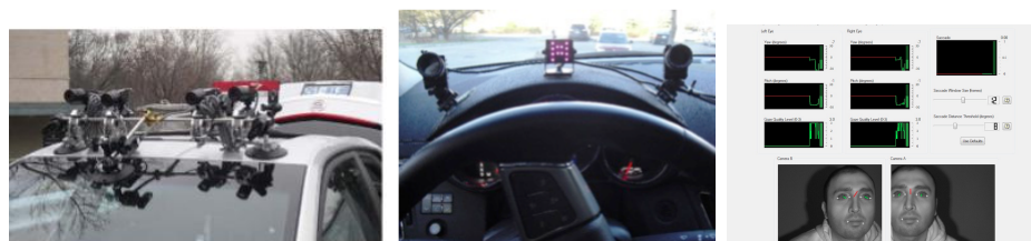
Figure 6.2: (left): Stereo vision system located on the vehicle's roof; (center): infrared gaze tracker; (right): FaceLAB system interface.
