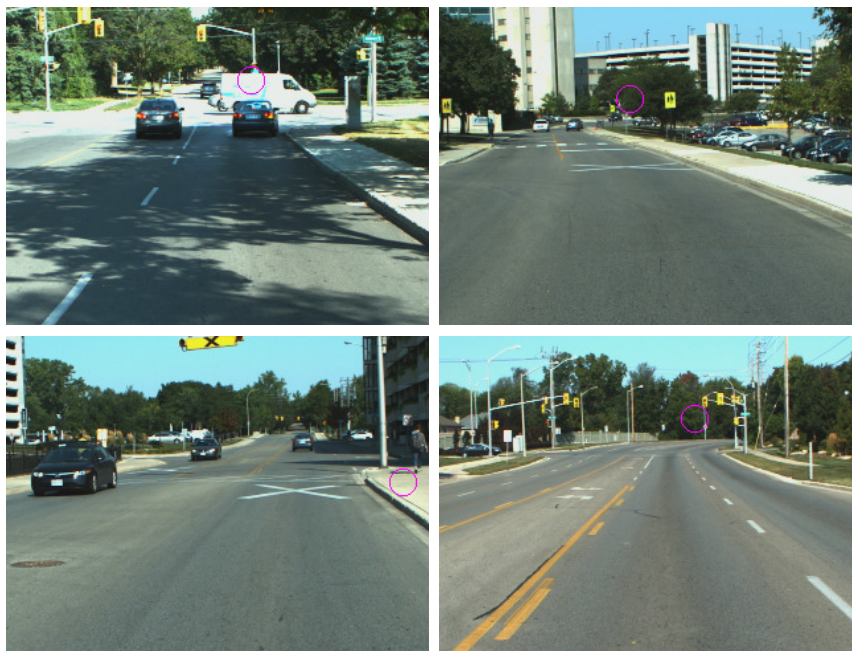
Figure 4.3: Various PoGs projected onto the forward stereo scene system of the vehicle, with less than 3-pixel movement in the last 15 frames (1/2 second)
