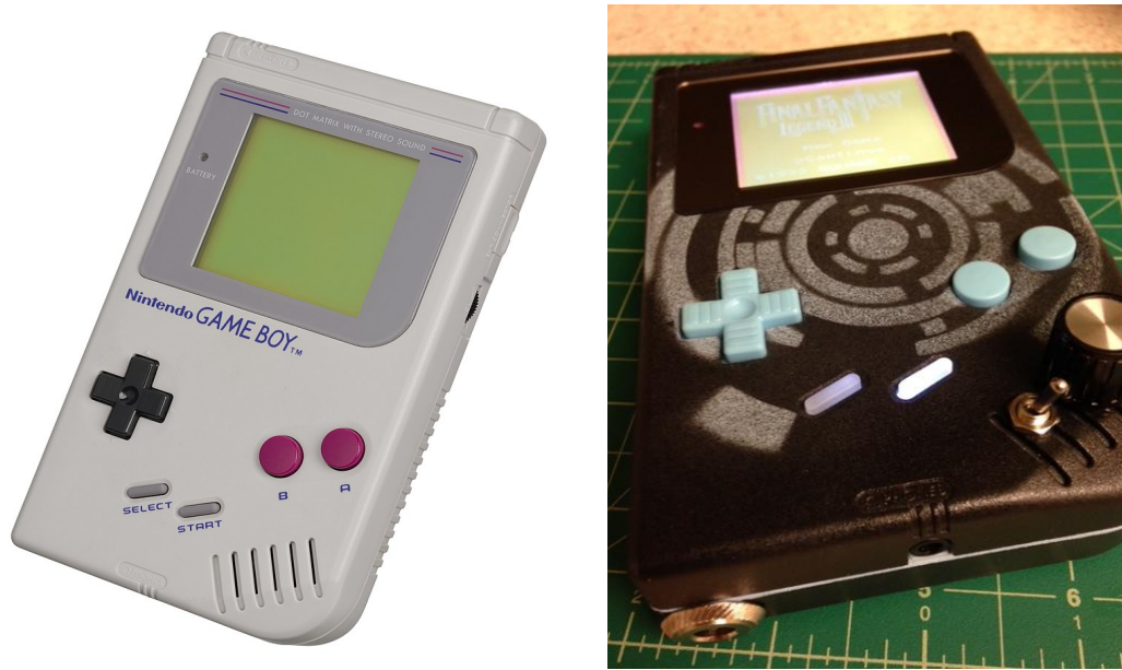
Figure 1. Left: An unmodified Nintendo Game Boy®. Right: A modified Game Boy that includes custom artwork on the case and buttons, LEDs behind the start and select buttons, an added audio port on the bottom left of the device that improves sound quality, and a switch and potentiometer that adjust the pitch of the device.
