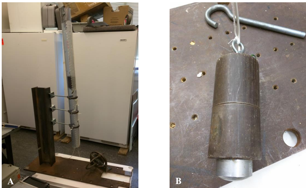
Figure 10. (A) Testing apparatus consisting of a vertical plastic tube with 0.2 m increments to measure drop height. (B) Impact device with a metal nose to deliver the impact force.
