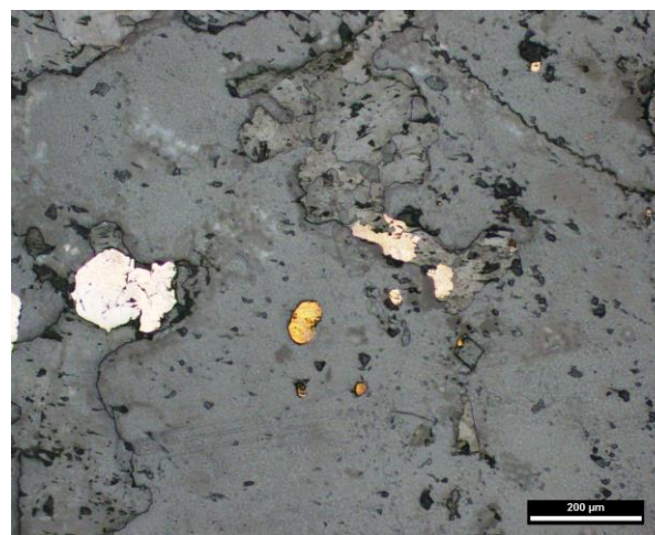
Figure 4. PPL reflected light, showing anhedral chalcopyrite (center), and arsenopyrite sides, scale at 200 \mu\text{m} .
