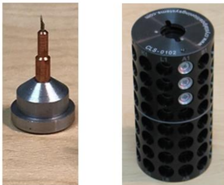
Figure 16. Illustrating SR-XRD sample preparation at Laboratory for Stable Isotope Science at Western University On the left a B3S ALS-style reusable goniometer base. On the right an SSRL-style sample cassette.
