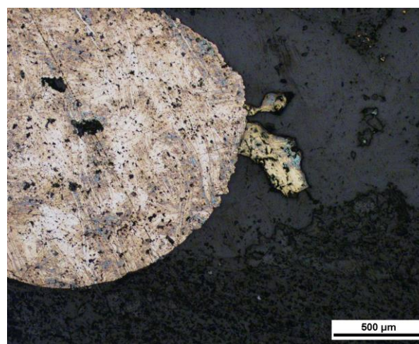
Figure 4. PPL reflected light, showing chalcopyrite (small right) and anhedral pyrite left, scale at 500 \mu\text{m} .
