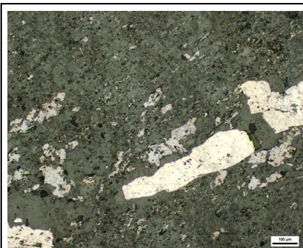
Figure 3. PPL reflected light, showing subhedral arsenopyrite grains and anhedral sphalerite grains in the greywacke, scale at 100 μm.
