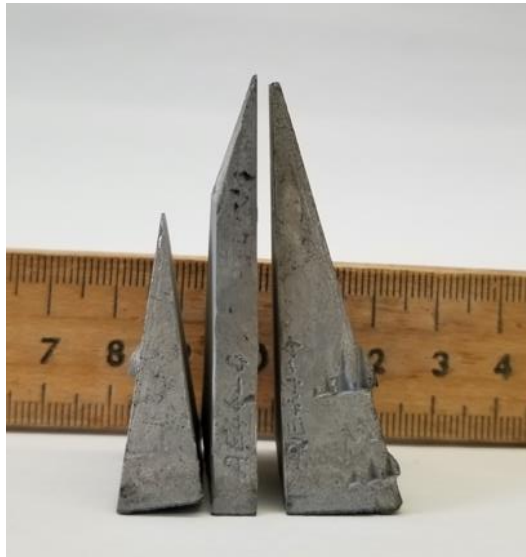
Figure 3.2.3 Illustration of a cast pyramidal specimen which has been sectioned to provide surfaces upon which micro-indentation tests were performed.
