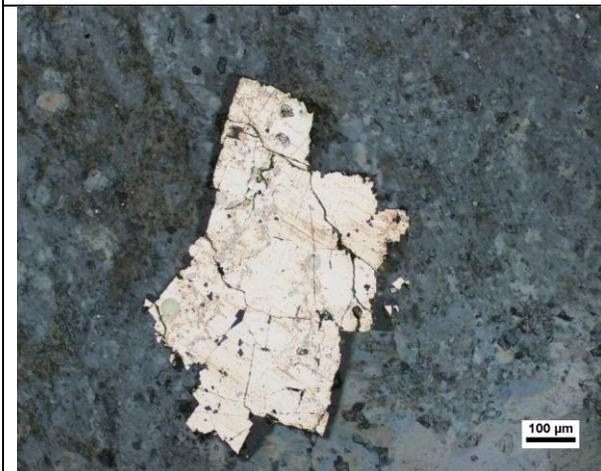
Figure 5. Fractured subhedral arsenopyrite in the groundmass (RL, X10).
