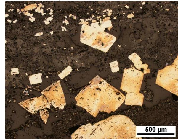
Figure 3. Corroded subhedral-euhedral coarse-grained pyrite grains and disseminated euhedral fine-grained arsenopyrite in carbonate vein (RL, 5X).
