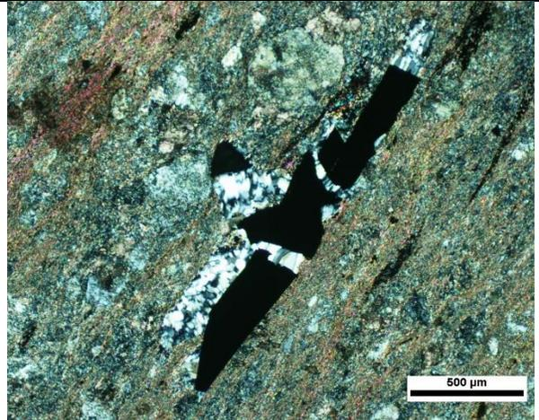
Figure 2. Fractured coarse-grained needle pyrite along with the foliation in the matrix. Recrystallized quartz formed pressure shadow texture around pyrite grains (XPL, 5X).
