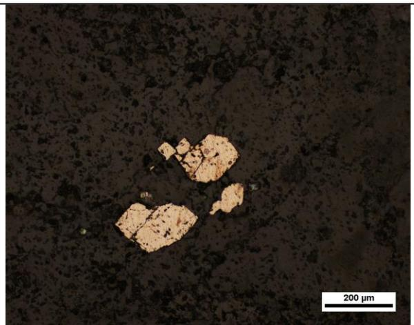
Figure 6. Corroded subhedral pyrite in quartz vein (RL, 20X)
