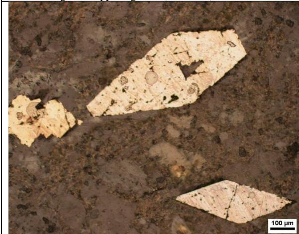
Figure 3. Corroded subhedral arsenopyrite with sphalerite inclusions in the pit sand fractures (RL, X10).
