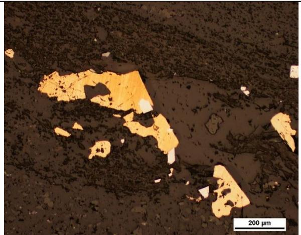
Figure 4. The combination of pyrite and arsenopyrite in the matrix (RL, X10).
