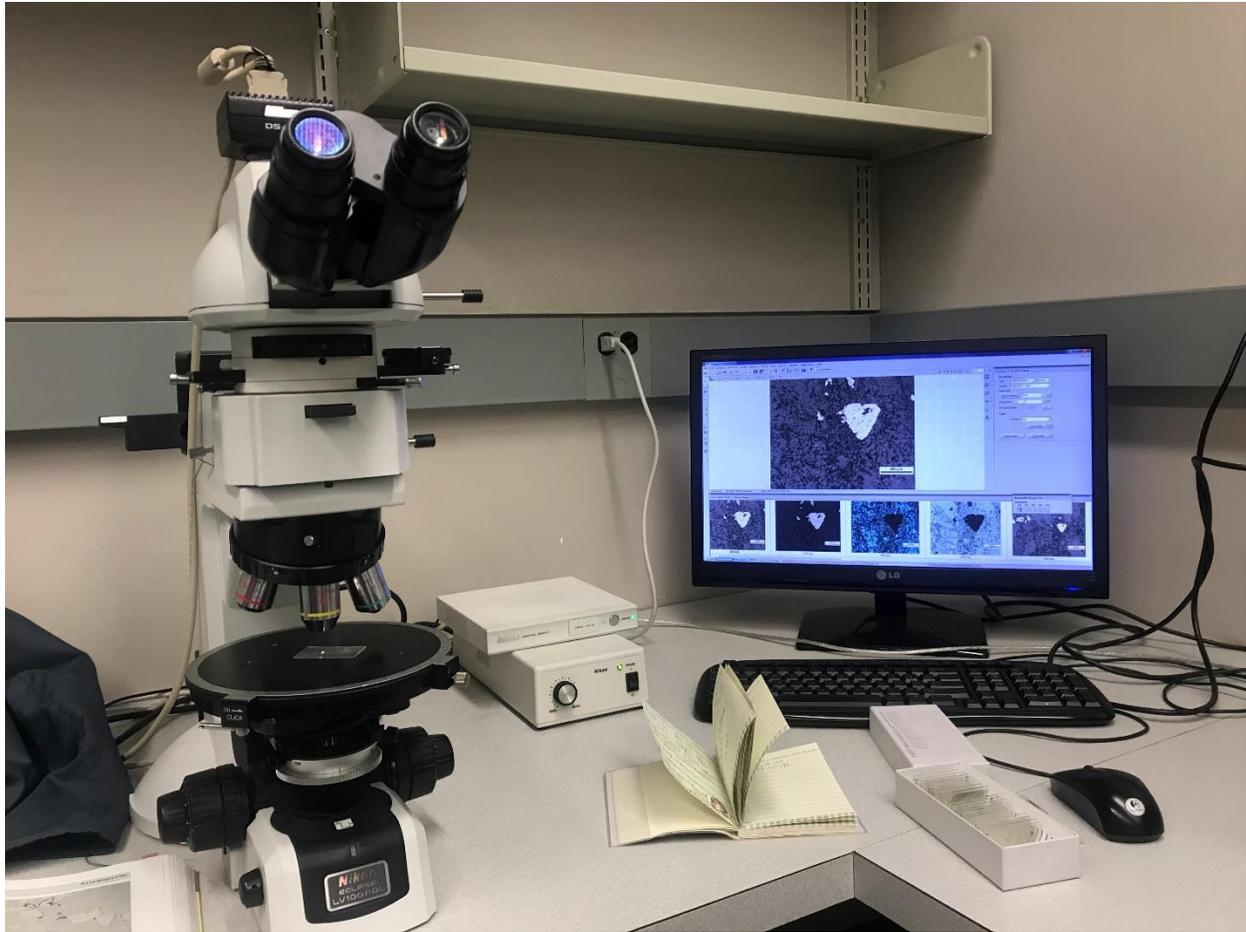
**Figure 3-2.** The Nikon LV100POL microscope mounted with Nikon DS-Ri1 digital camera used for petrographic analysis in the Earth and Planetary Materials Analysis Laboratory at Western University.
