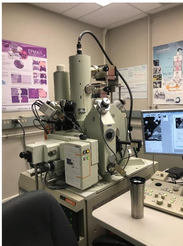
**Figure 3-18.** The JEOL JXA-8530F field-emission electron microprobe, at the Earth and Planetary Materials Analysis Laboratory, at Western University.
