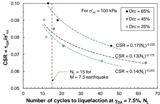
Figure 12. CSR versus number of cycles ( $N_L$ ) to trigger liquefaction for Boler sand at  $\sigma'_{vc} = 100$  kPa
