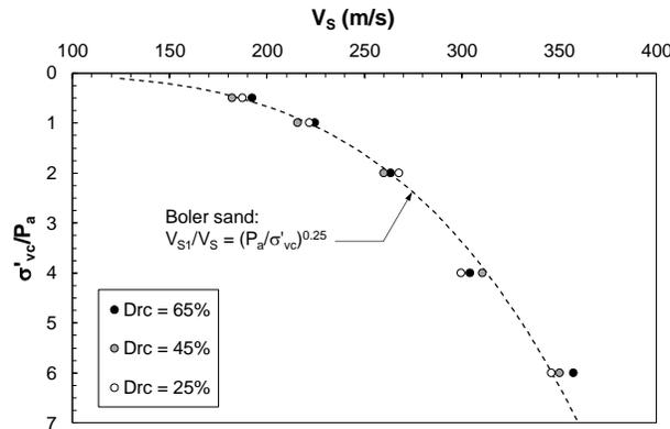
Figure 5. Variation of  $V_s$  with normalized effective vertical stress ( $\sigma'_{vc}/P_a$ ) for Boler sand specimens
