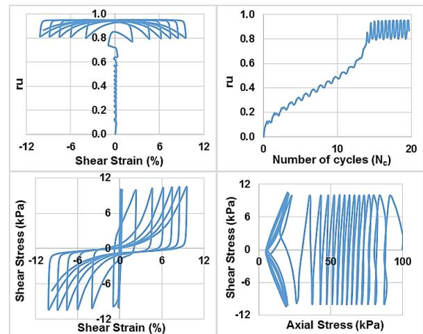
Figure 11. Cyclic DSS test results on a Boler sand specimen at  $D_{rc} = 65\%$ ,  $\sigma'_{vc} = 100$  kPa and  $CSR = 0.100$
