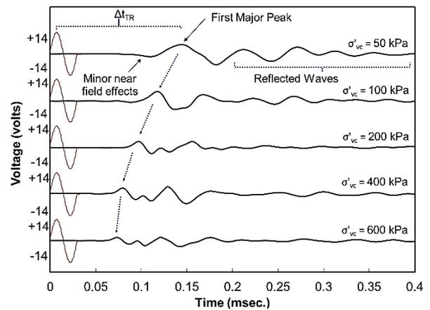
Figure 4. Shear wave signals for  $D_{rc} = 45\%$  specimen
