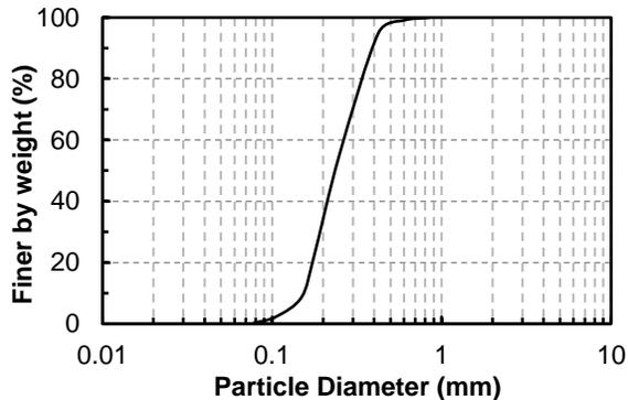
Figure 1. Average grain size distribution of Boler sand
