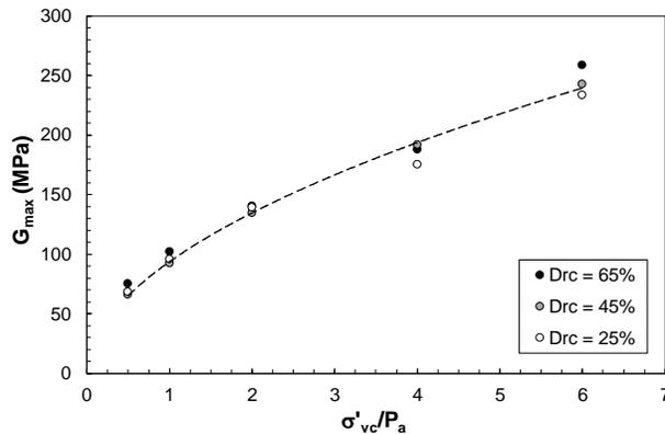
Figure 9. Variation of  $G_{max}$  with  $\sigma'_{vc}$  for Boler sand at  $D_{rc} = 25, 45,$  and  $65\%$
