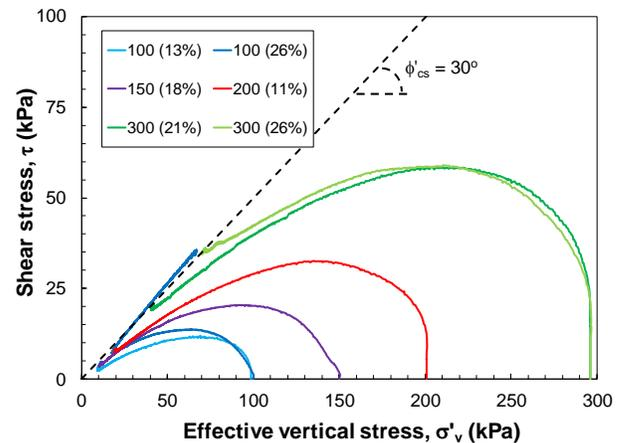
Figure 2. Stress paths for some of the constant-volume monotonic DSS tests
