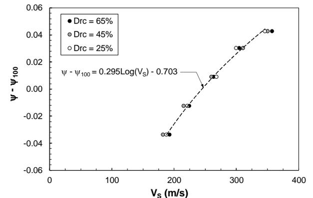
Figure 8.  $V_s$  versus ( $\psi - \psi_{100}$ ) from the DSS tests of this study.  $\psi_{100}$  is the state parameter at  $\sigma'_{vc} = 100$  kPa
